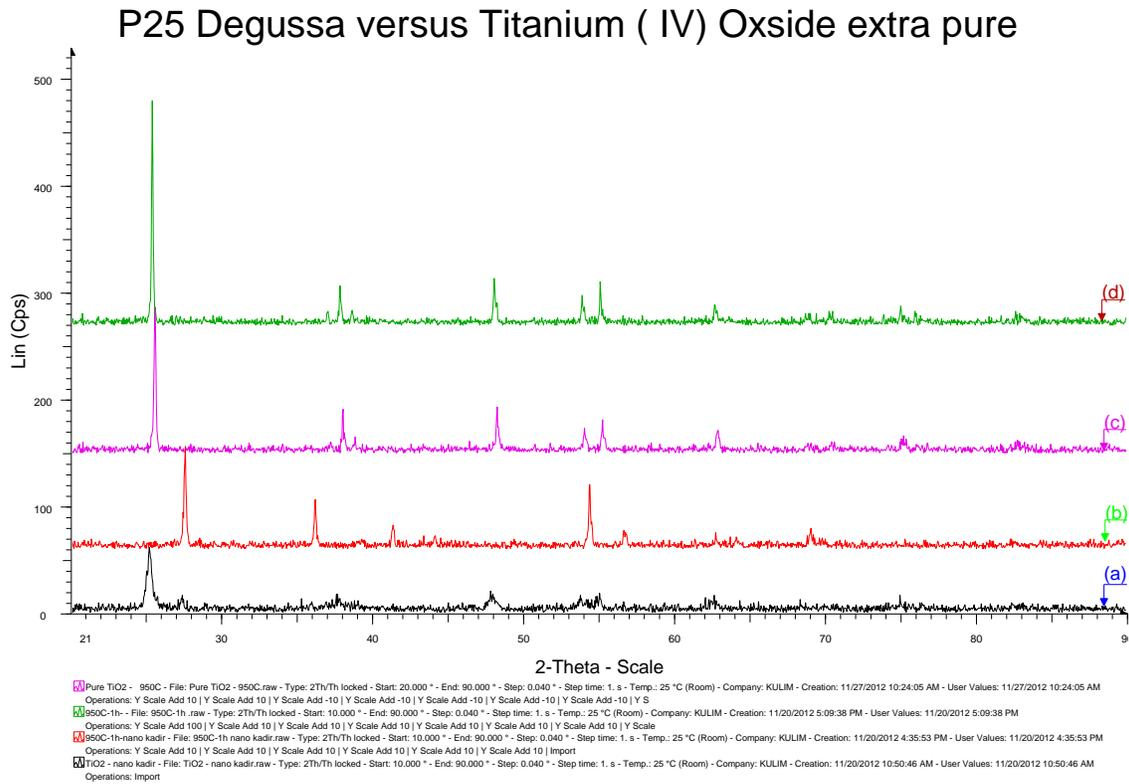
Figure 3: XRD patterns of the samples; (a) raw (anatase 75%, rutile 25%) Degussa P25; (b) Degussa P25 after calcining at 950 °C, and turns to rutile completely; (c) (anatase  $\text{TiO}_2$ ) undoped sample after calcining at 950°C; and (d) ( $\text{TiO}_2 + \text{talc}$ ) doped sample after 950°C shows increasing anatase intensity
