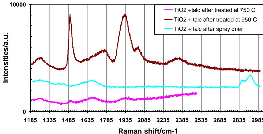
Figure 5: Raman shift of the (TiO<sub>2</sub>+ talc) doped sample before and after calcination
