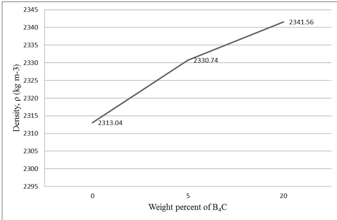
Figure 1: Effects of B<sub>4</sub>C addition on the density of concrete
