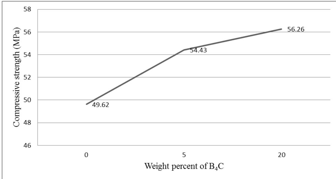
Figure 2: Effects of B<sub>4</sub>C addition on the compressive strength of concrete
