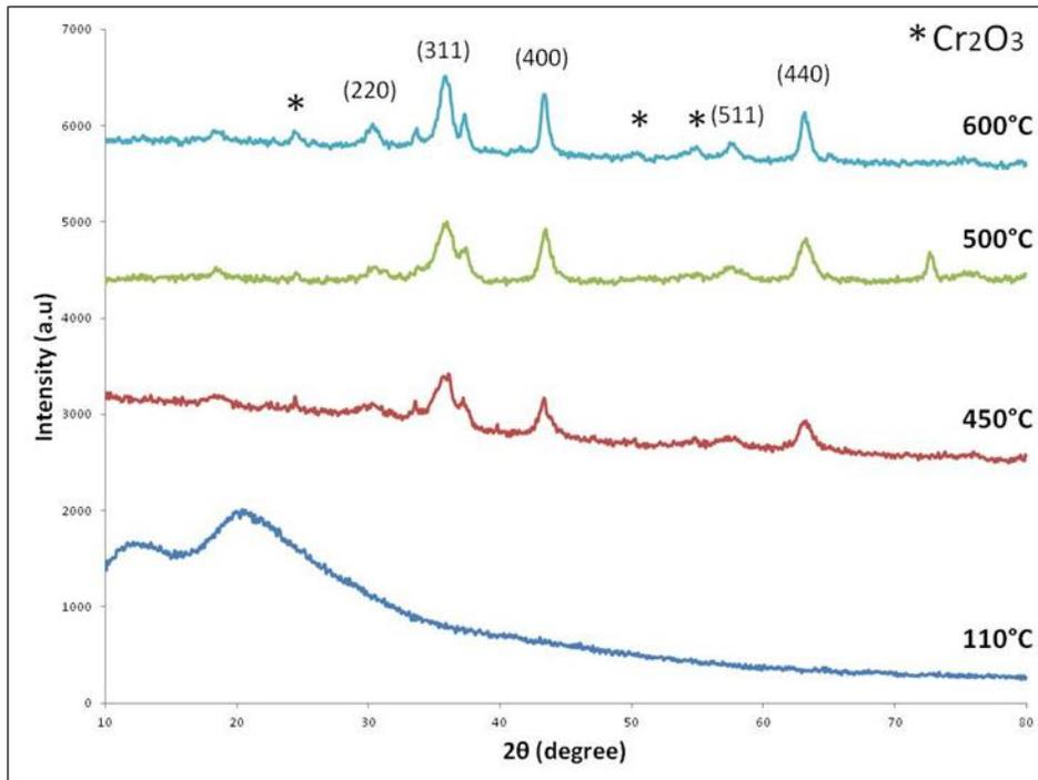
Figure 2: XRD patterns of NiCr<sub>2</sub>O<sub>4</sub> calcined at difference temperatures
