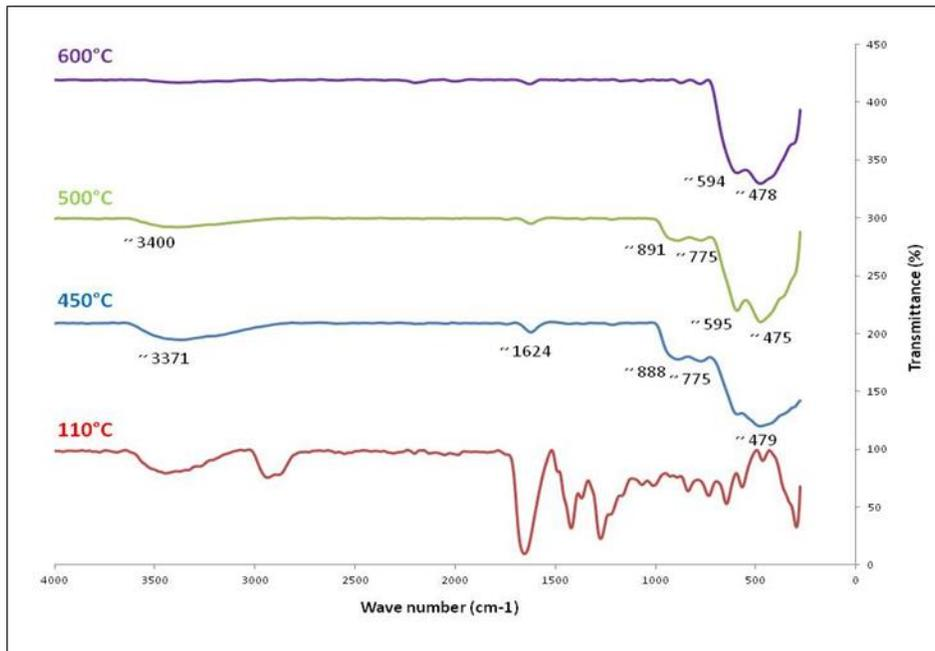
Figure1: FT-IR spectra of NiCr<sub>2</sub>O<sub>4</sub> calcined at difference temperatures
