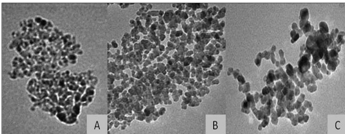
Figure 3: TEM images of nickel chromite calcined at (A) 450°C, (B) 500°C and (C) 600°C in a range of 100 nm
