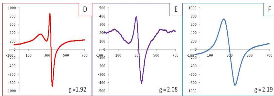
Figure 4: ESR spectra of nickel chromite calcined at (D) 450°C, (E) 500°C and (F) 600°C
