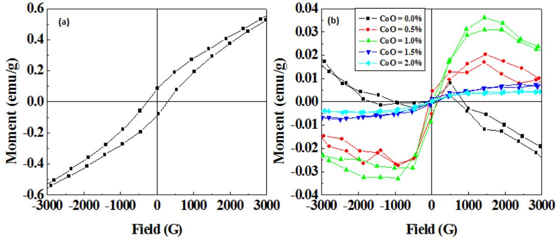
Figure 2: (a) Magnetic hysteresis loops of pure CoO NPs (b) samples of  $(69-x)\text{P}_2\text{O}_5-10\text{MgO}-20\text{ZnCl}_2-1\text{Er}_2\text{O}_3-(x)\text{CoO}$  with  $x = 0.0, 0.5, 1.0, 1.5$  and  $2.0$
