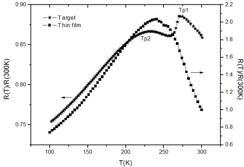
Figure 2: Normalised resistance via temperature of the LCMO film and target
