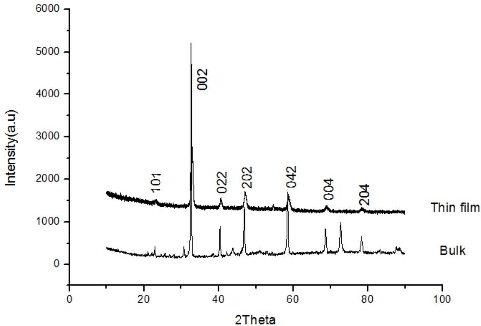
Figure 1: X-ray diffraction pattern of the  $\text{La}_{5/8}\text{Ca}_{3/8}\text{MnO}_3$  for film and PLD target
