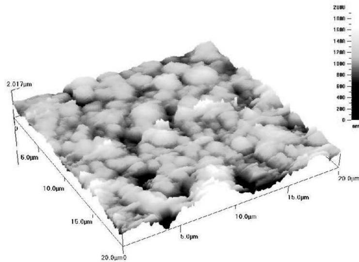
Figure 4: AFM Micrograph for  $\text{La}_{5/8}\text{Ca}_{3/8}\text{MnO}_3$  polycrystalline film
