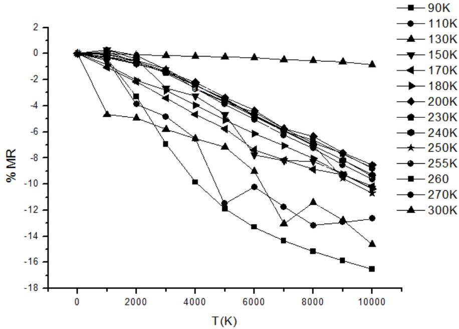
Figure 3: %MR curves as a function of applied magnetic field at various temperatures for LCMO/Si film
