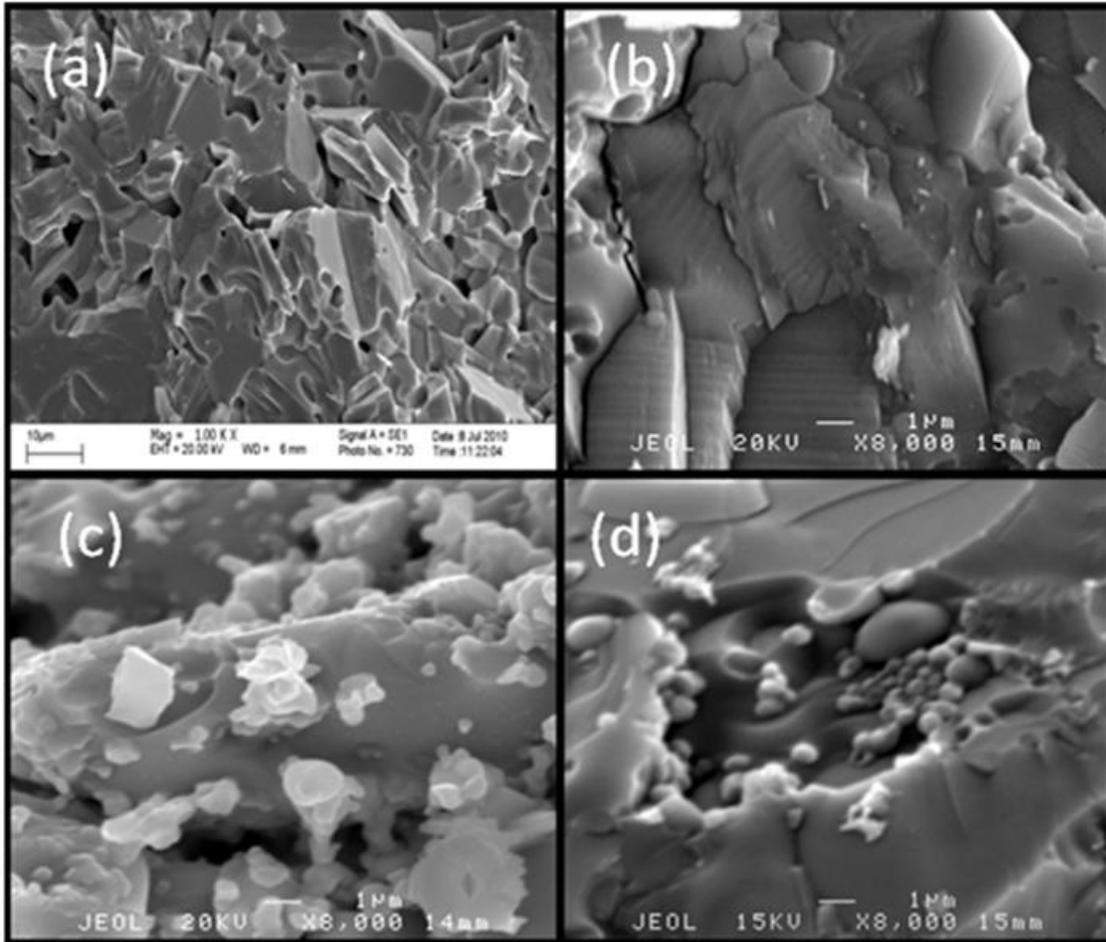
Figure 6: SEM micrographs of the (a) pure samples and samples reacted with (b) 0.5 wt.%, (c) 1.0 wt.% and (d) 2.0 wt.% of nano-SiC
