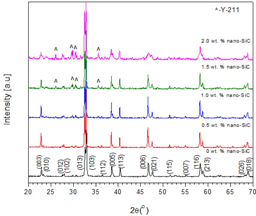
Figure 1: X-ray powder diffraction patterns of  $\theta - 2\theta$  scan
