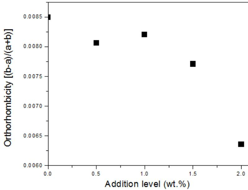
Figure 3: Dependency of orthorhombicity on nano-SiC addition
