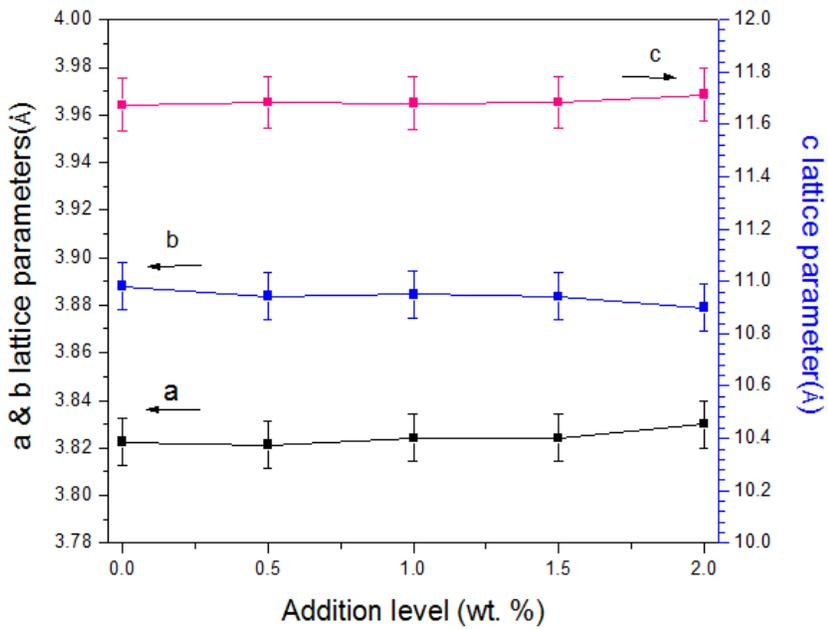
Figure 2: Evolution of lattice parameters with the addition level of nano-SiC
