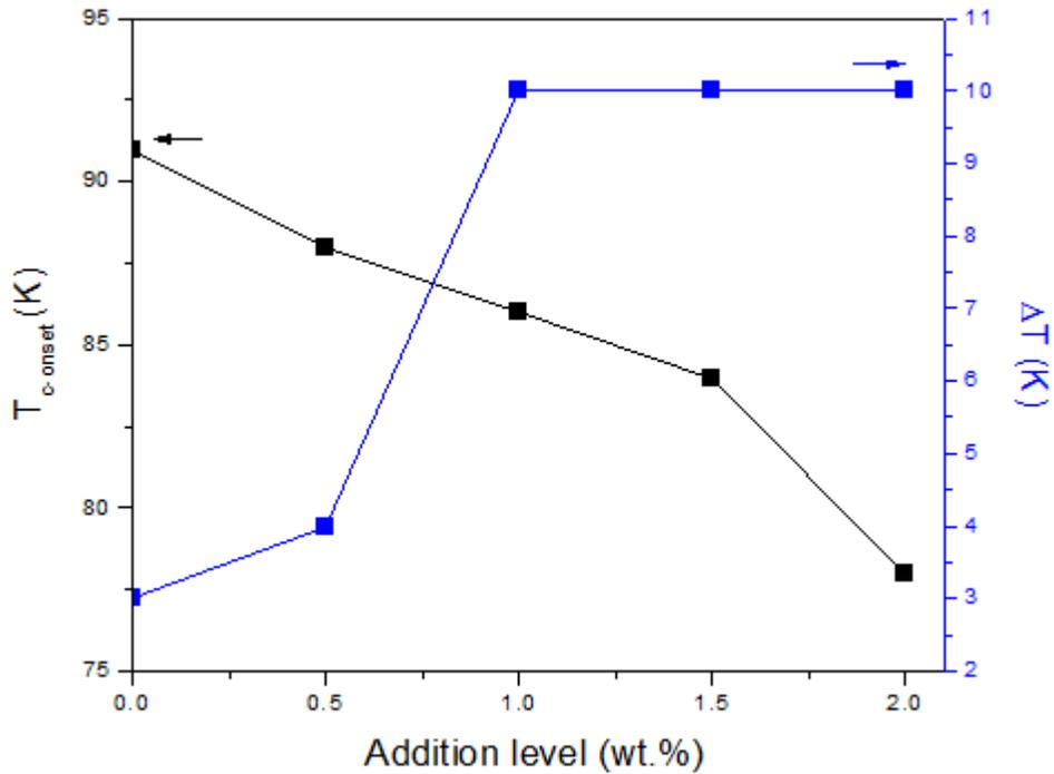
Figure 5: Variation of  $T_{c-onset}$  and  $\Delta T$  with addition of nano-SiC. Lines are guides for the eyes only
