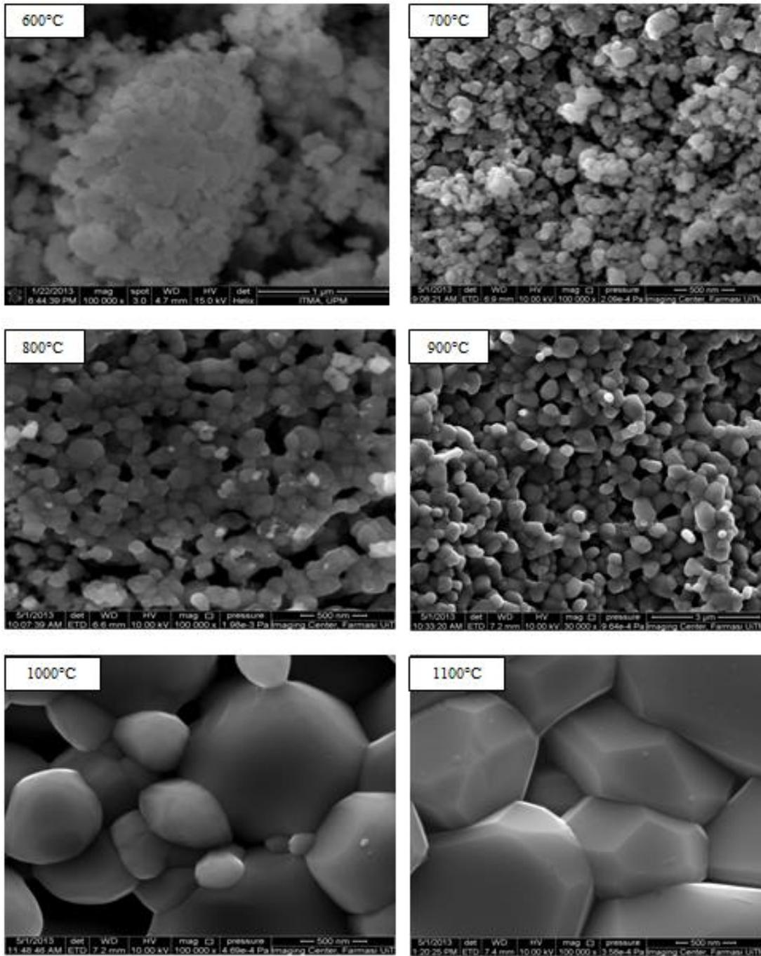
Figure 4: Microstructures of MgZnCu ferrites at various temperatures
