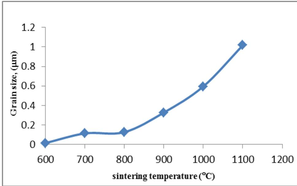
Figure5: Average grain size versus sintering temperatures
