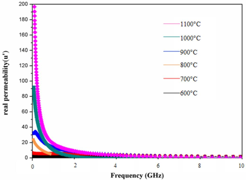
Figure 2: A graph of initial permeability against frequency
