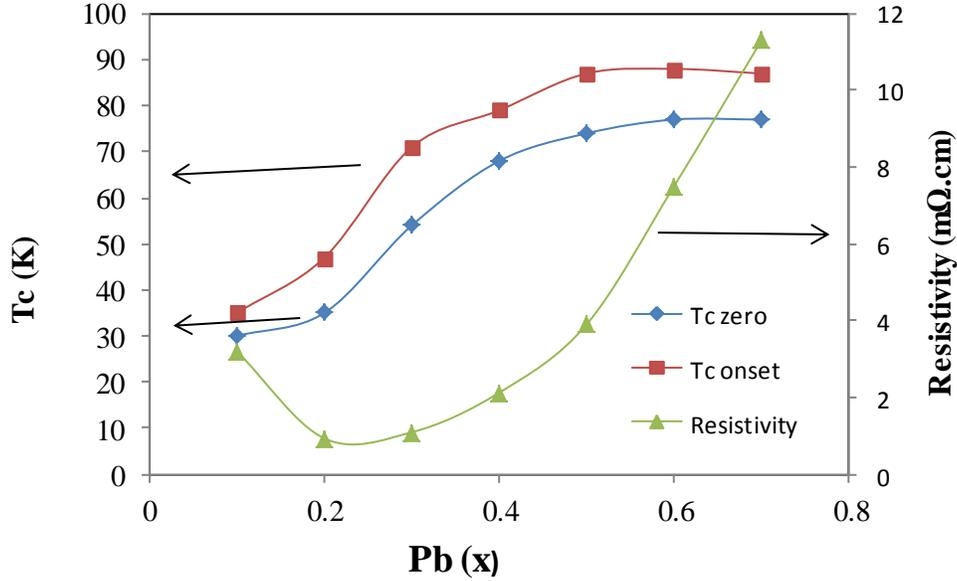
Figure 3: Normal state electrical resistivity at 300 K and the variation of  $T_{c \text{ onset}}$  and  $T_{c \text{ zero}}$  as function of  $(\text{Tl}_{1-x}\text{Pb}_x)\text{Sr}_2\text{CaCu}_2\text{O}_{7-\delta}$
