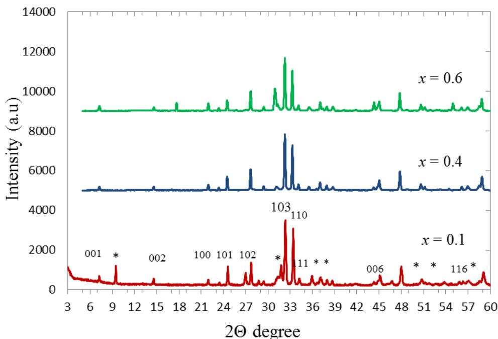
Figure 1: Powder X-ray diffraction patterns for  $(\text{Tl}_{1-x}\text{Pb}_x)\text{Sr}_2\text{CaCu}_2\text{O}_{7-\delta}$   $x = 0.1, 0.4$  and  $0.6$ . (\*) indicates the Tl-1201 phase
