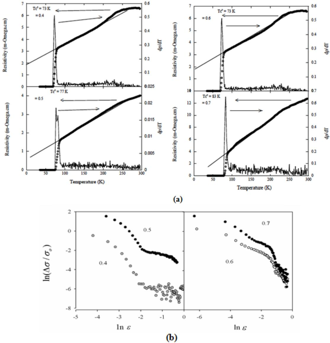
Figure 4: (a) Electrical resistivity vs. temperature plot with extrapolated linear fit and  $(d\rho/dT)$ , residual resistivity  $\rho_0$  and (b) the  $\ln(\Delta\sigma/\sigma_0)$  versus  $\ln(\epsilon)$  plot with the exponent ( $\lambda_2$  and  $\lambda_3$ ) values gives the excess conductivity behaviour of  $(Tl_{1-x}Pb_x)Sr_2CaCu_2O_{7-\delta}$  with  $x = 0.4, 0.5, 0.6$  and  $0.7$
