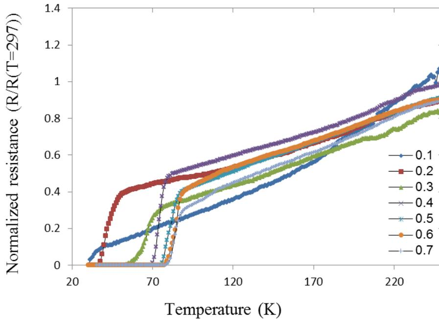
Figure 2: The temperature dependence of the resistance of  $(\text{Tl}_{1-x}\text{Pb}_x)\text{Sr}_2\text{CaCu}_2\text{O}_{7-\delta}$  for  $x = 0.1, 0.2, 0.3, 0.4, 0.5, 0.6$  and  $0.7$
