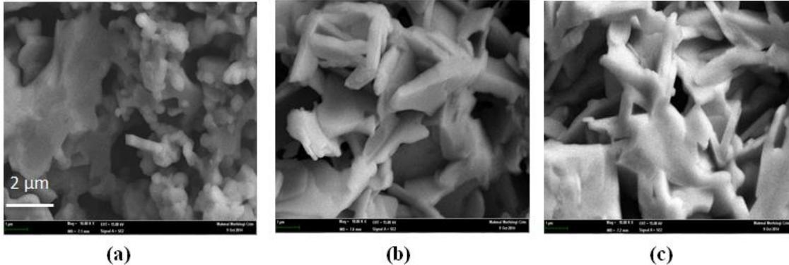
Figure 5. Scanning electron micrographs (at 15Kv) for  $(\text{Tl}_{1-x}\text{Pb}_x)\text{Sr}_2\text{CaCu}_2\text{O}_{7-\delta}$  for (a)  $x = 0.1$ , (b)  $x = 0.4$  and (c)  $x = 0.6$
