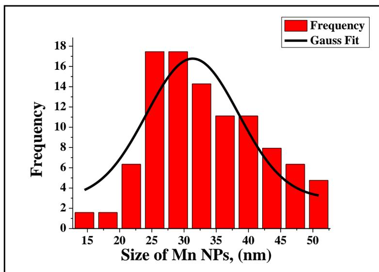
Figure 5: Gaussian fit of sizes distribution Mn NPs
