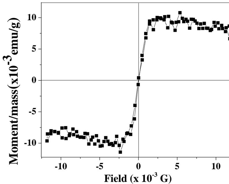
Figure 3 (b) : Hysteresis loop for glasses with and without Mn NPs.
