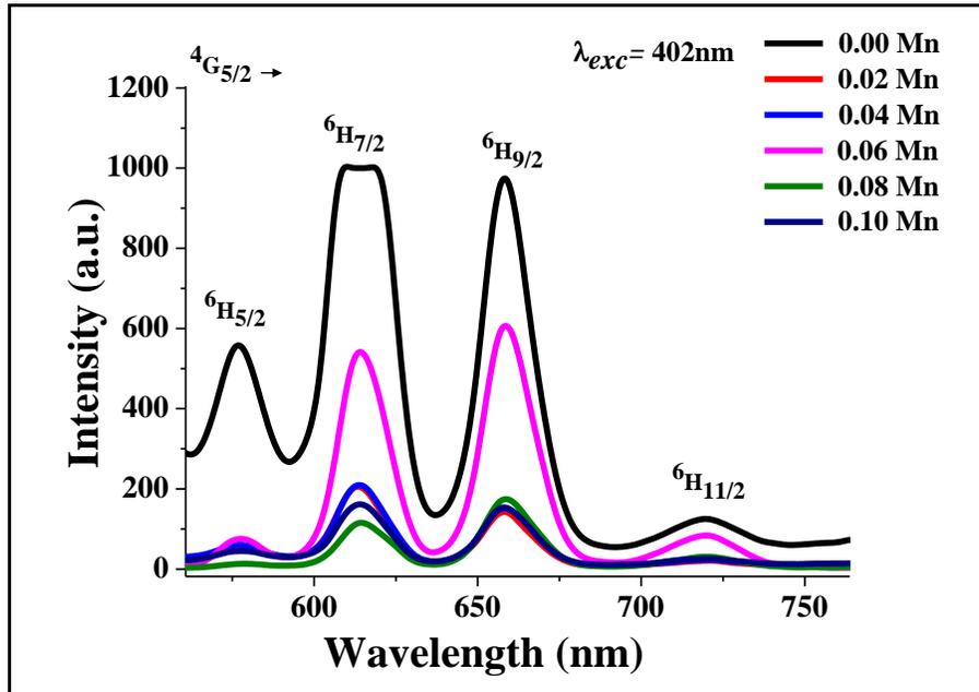
Figure 2: NPs concentration dependent emission spectra for all samples
