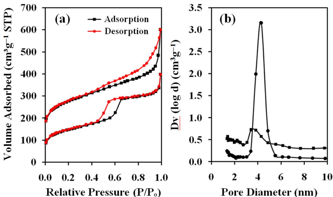
Figure 1: The nitrogen adsorption–desorption isotherms (a) and pore size distribution (b) of SBA-15 and OMC
