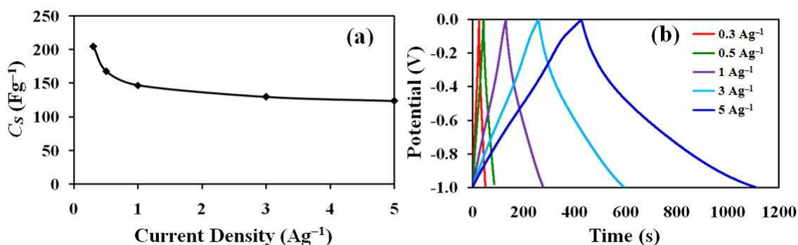
Figure 5: The specific capacitance ( $C_s$ ) of OMC as a function of discharging current density (a) and charge-discharge curves of OMC at 0.3, 0.5, 1, 3, and 5  $Ag^{-1}$  (b)
