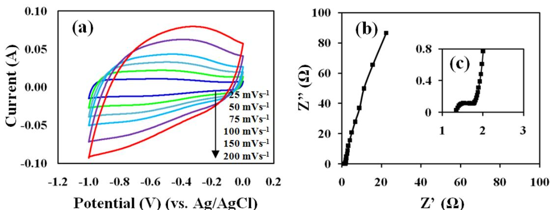
Figure 4: Cyclic voltammograms of OMC at (inner to outer) 25, 50, 75, 100, 150, and 200  $\text{mVs}^{-1}$  (a) and Nyquist plot (b). The inset (c) shows the high frequency region of impedance
