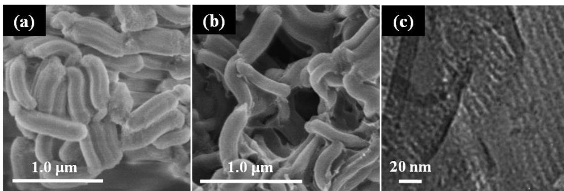
Figure 3: The FESEM images of SBA-15 (a), OMC (b); and TEM image of OMC (c)
