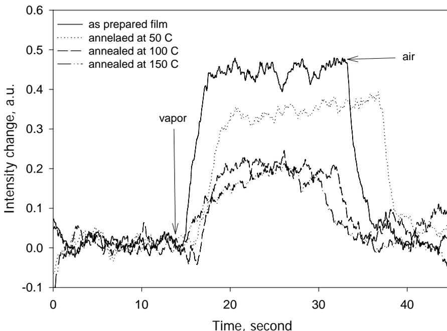
Figure 6. The comparison of the sensing sensitivity of the as prepared thin film and the annealed films.
