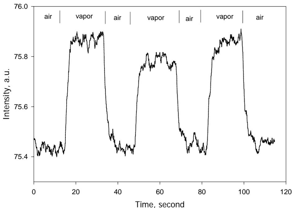
Figure 5. The sensing sensitivity of the CoTPP films towards the presence of saturated vapor of cyclohexane which was recorded at the wavelength of 626 nm, the light source.
