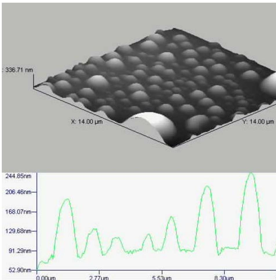
Figure 3. The AFM image and the cross sectional analysis of ABPCA film.
