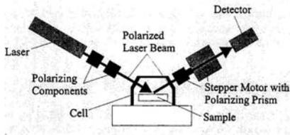
Fig.1: Principle of Minsearch-Ellipsometer
