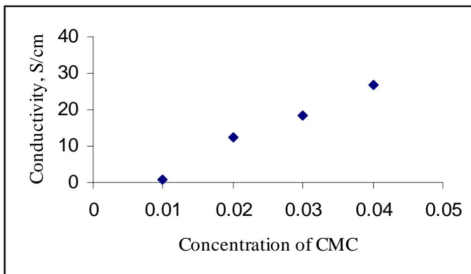
Figure 1. Conductivity of PPY-CMC vs. concentration of CMC.
