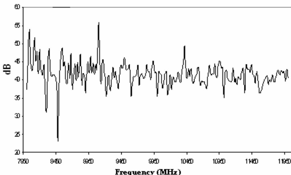
Figure 4. The electromagnetic shieldeffectiveness of PPY-CMC in the frequency range of 8-12 GHz.
