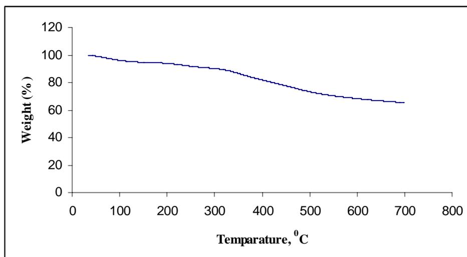
Figure 7. Thermogravimetric analysis of PPY-PVA film.
