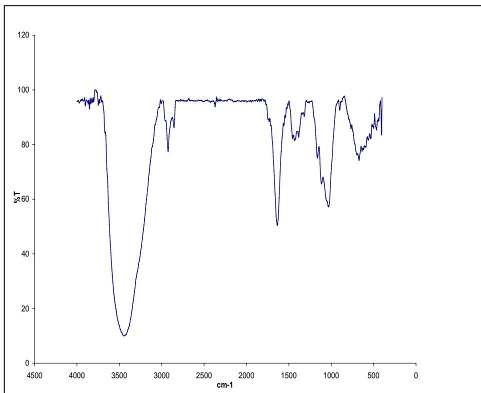
Figure 2. The FT-IR spectra of PPY-CMC composite film.
