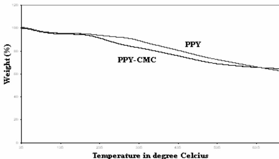
Figure 3. Thermogravimetric analysis of PPY-CMC film.
