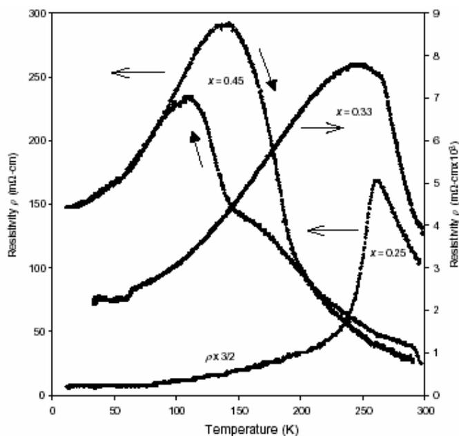
Figure 1. Resistivity versus temperature curves for  $\text{La}_{1-x}\text{Ca}_x\text{MnO}_3$  with  $x = 0.25, 0.35$  and  $0.45$  [26].
