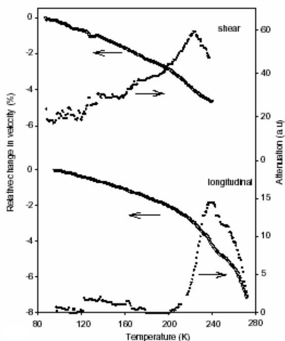
Figure 2. Temperature-dependence of longitudinal and shear velocities with their attenuation of  $\text{La}_{1-x}\text{Ca}_x\text{MnO}_3$  for  $x = 0.33$  [26].
