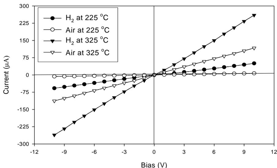
Fig. 1. I-V characteristics of 2SnO<sub>2</sub>:3CuO at 225 °C and 325 °C in air and 200 ppm H<sub>2</sub>, respectively.
