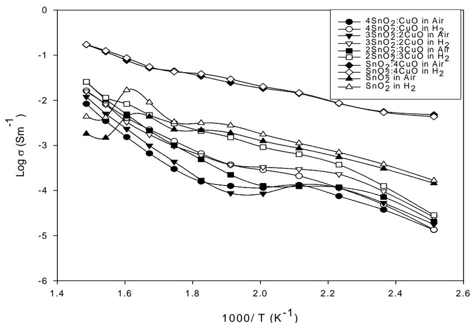
Fig. 2. Temperature dependence of electrical conductivity of the single oxide SnO<sub>2</sub> and SnO<sub>2</sub>-CuO composites in air and 200 ppm H<sub>2</sub>.
