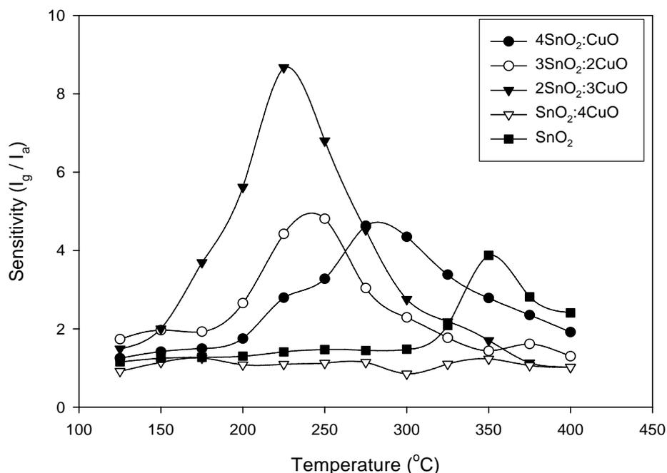
Fig. 3. Temperature dependence of H<sub>2</sub> sensitivity (200 ppm) of SnO<sub>2</sub>-CuO composites.
