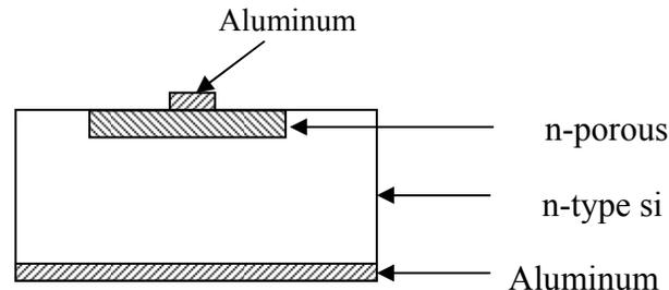
Figure 1: Sectional-view of the final device.
