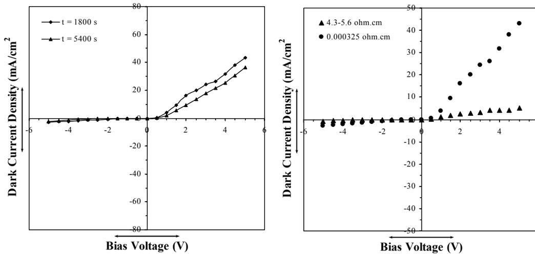
Figure (2): I-V characteristics of Al/PS/n-Si/Al structure at 1800 s etching time for two used resistivities.
