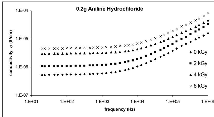
Figure 2: Variation of conductivity with frequency of PVA/PANI for 0.2 g Aniline hydrochloride
