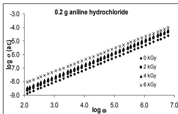
Figure 5: log-log plot of ac conductivity vs. frequency at various doses for 0.2g aniline hydrochloride
