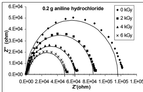
Figure 3: Complex impedance Nyquits plot at different dose for 0.2g aniline hydrochloride
