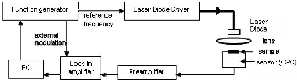
Figure 1. Schematic diagram of the experimental set-up
