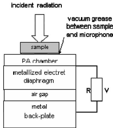
Figure 2. Cross-section of the OPC
