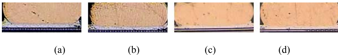
Figure 3: Optical microscopy image of a typical gold ball cross-section without HTS test: (a) power 19% and force 970 Nm, (b) power 24% and force 790 Nm, (c) power 24% and force 970 Nm, (d) power 19% and force 790 Nm.
