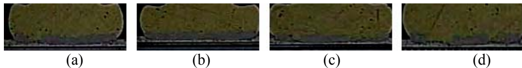
Figure 5: Optical microscopy image of a typical gold ball cross-section with HTS test at 175°C for 384 hours (a) power 19% and force 970 Nm (b) power 24% and force 790 Nm (c) power 24% and force 970 Nm (d) power 19% and force 790 Nm.
