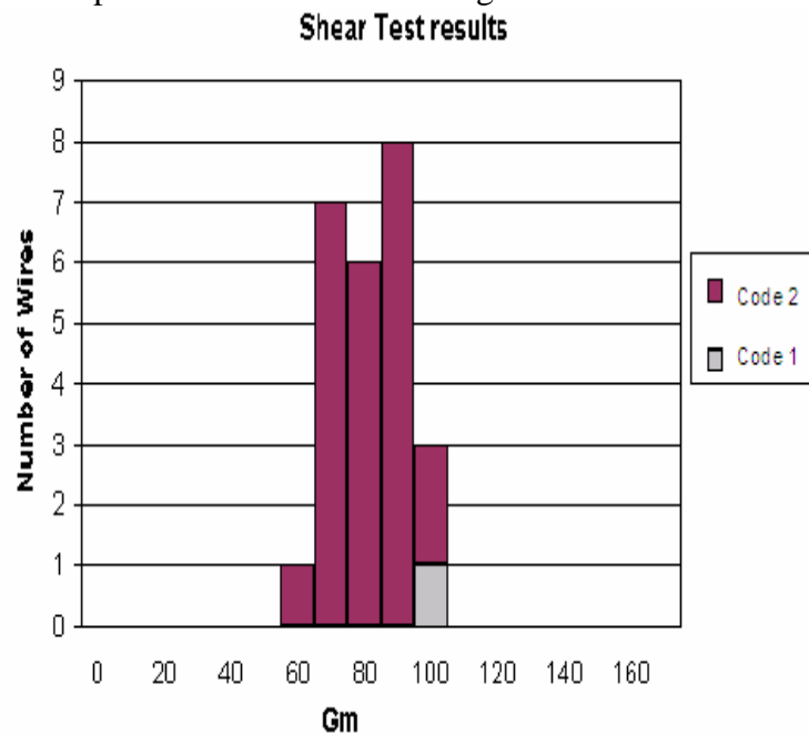
Figure 5: Ball shear results after aging at 150°C for 500 hours.
