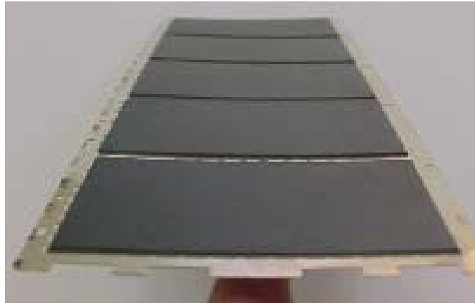
Figure 7: QFN strip showing the 'smiling face' (edge up) orientation.
