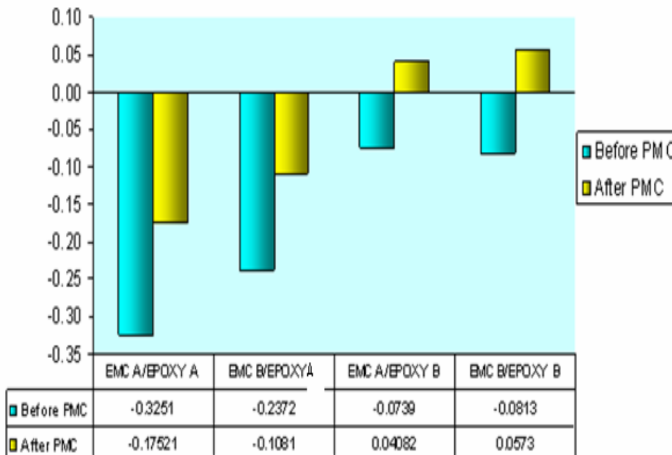
Figure 5: Package warpage before PMC and after PMC.
