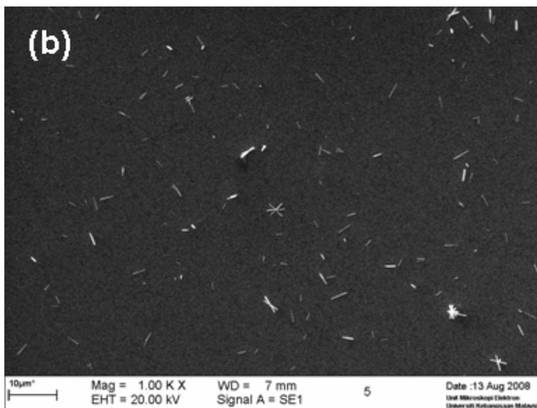
Figure 3: SEM images of ZnO rods formed on (a) ITO substrate and (b) unannealed ZnO seed layer.
