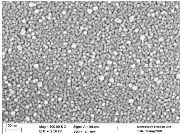
Figure 1: SEM images of ZnO seed layer annealed at 300 °C
