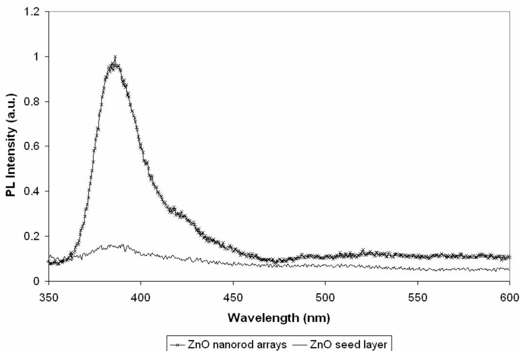
Figure 5: Room temperature photoluminescence spectra of ZnO nanorod arrays and ZnO seed layer
