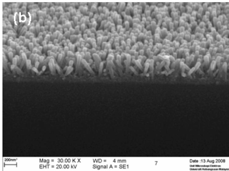
Figure 2: a) Top-view and b) cross-sectional SEM images of ZnO nanorod arrays grown on seeded-ITO substrate
