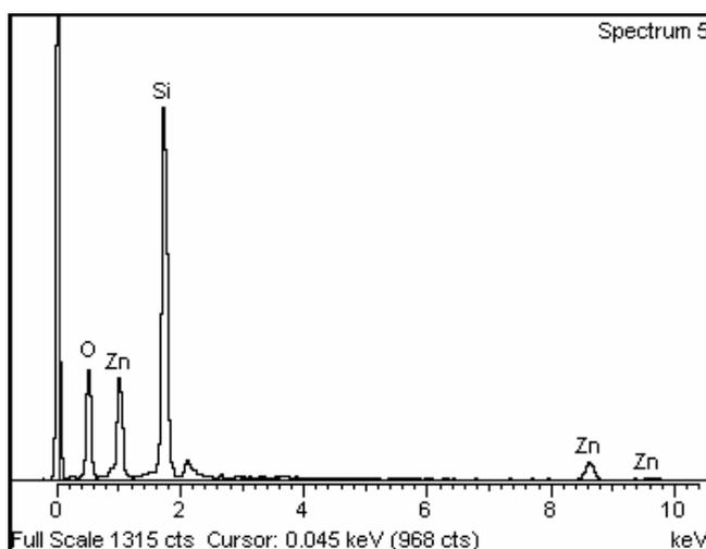
Figure 4: EDX spectrum of the ZnO nanorods grown on seeded-quartz substrate
