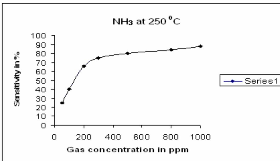
Figure 5: Variation of gas sensitivity with gas concentration.
