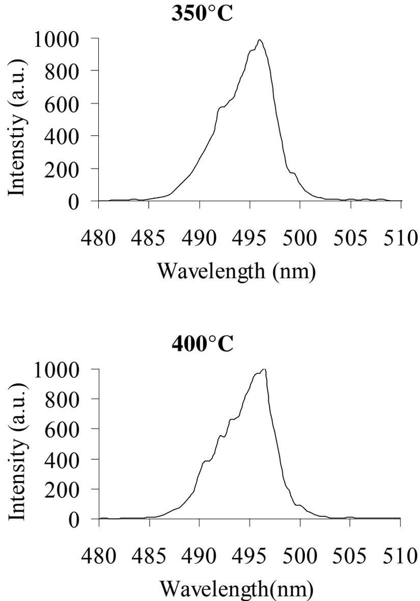
Figure 4: PL spectra of ZnS thin film for different annealing temperature
