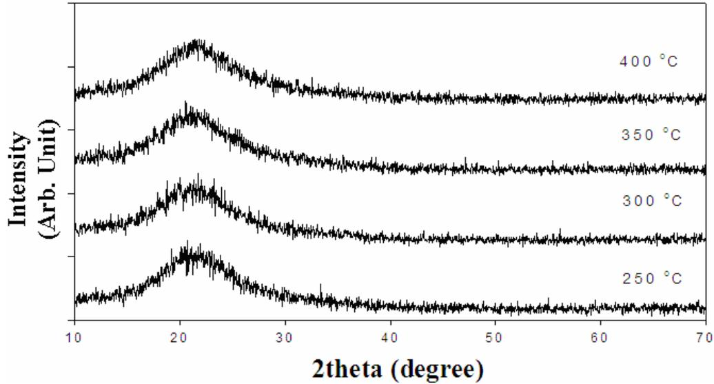
Figure 1: X-ray diffraction pattern of ZnS produced by annealing at 250°C, 300°C, 350°C and 400°C
