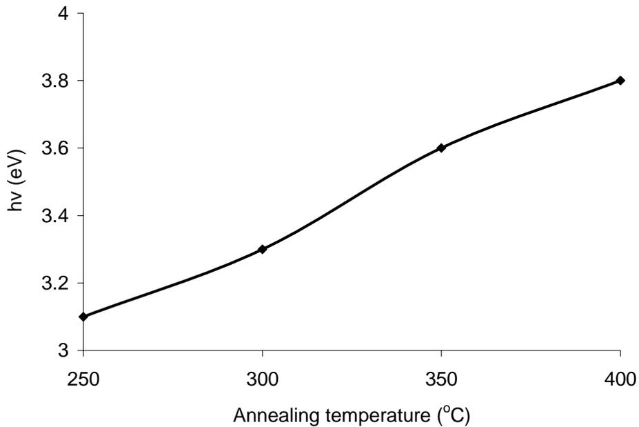
Figure 5: Relation between annealing temperature and band gap energy.
