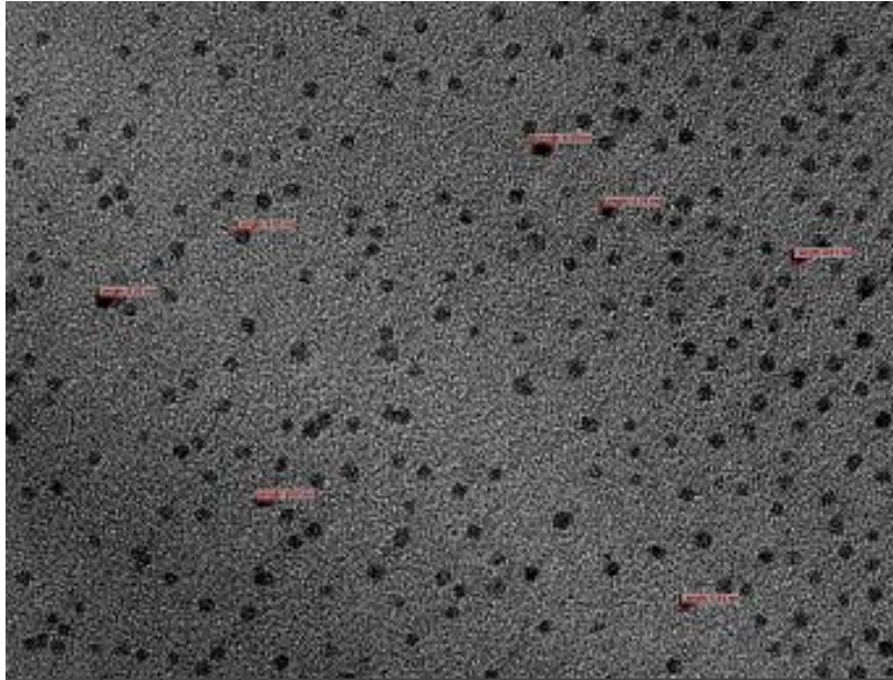
Figure 2: Shows the TEM images of the CdTe QDs that was taken from the sample grown for 25 s.
