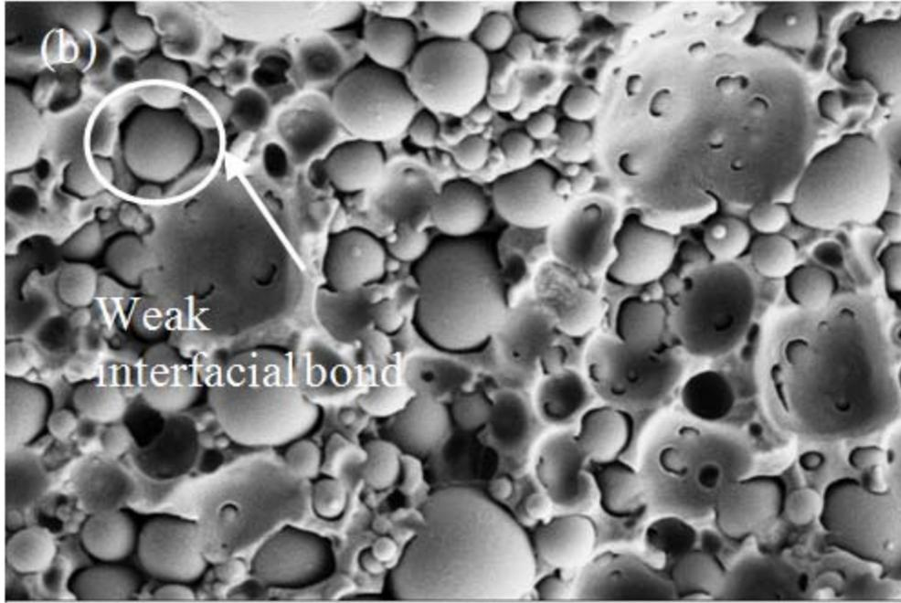
Figure 4: SEM micrographs of flexural surface of (a) EMC control and (b) EMC modified with 5wt% loading of PMMA-grafted NR
