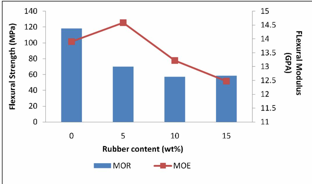
Figure 1: Effect of PMMA-grafted NR loading on flexural strength and modulus of EMC filled spherical fused silica
