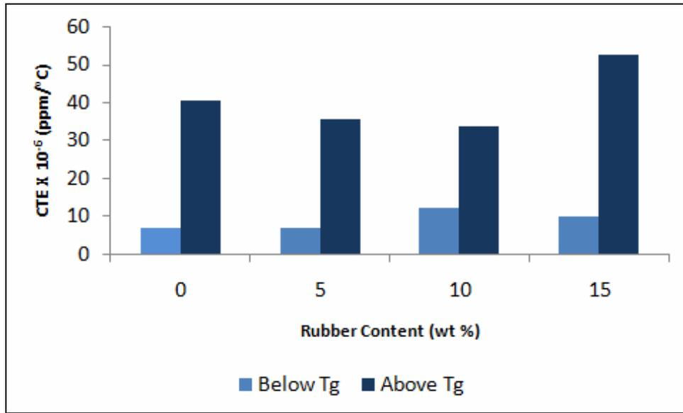
Figure 3: CTE of EMCs with different rubber content
