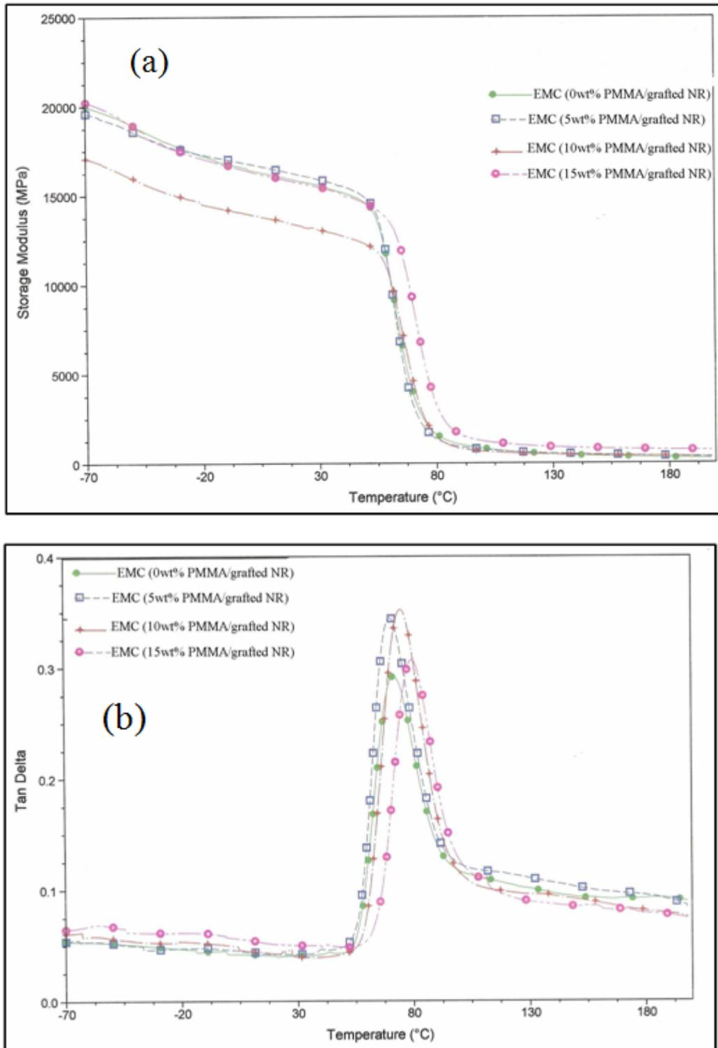
Figure 2: (a)  $E'$  and (b)  $\tan \delta$  of EMC modified with PMMA-grafted NR and control EMC
