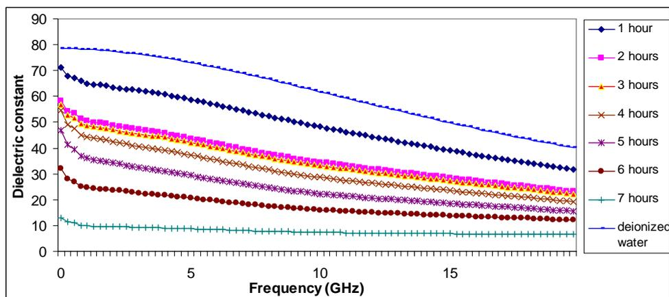
Figure 3: Dielectric constant of turmeric as a function of frequency with respect to the drying hours
