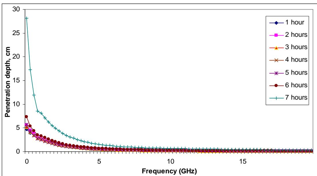
Figure 6: Penetration depth of turmeric as a function of frequency with respect to the drying hours
