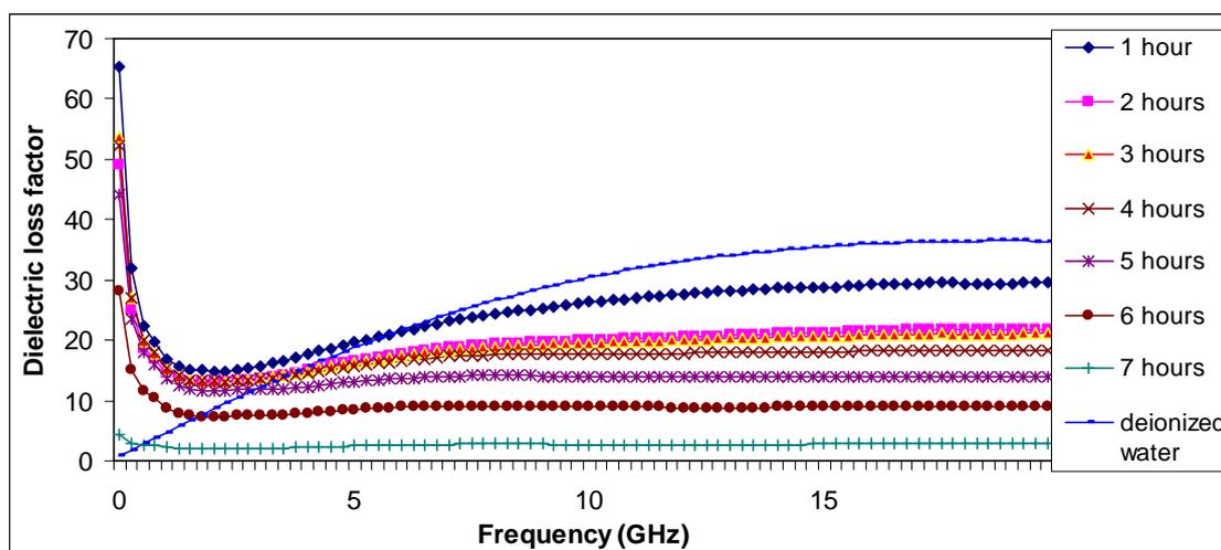
Figure 4: Dielectric loss factor of turmeric as a function of frequency with respect to the drying hours
