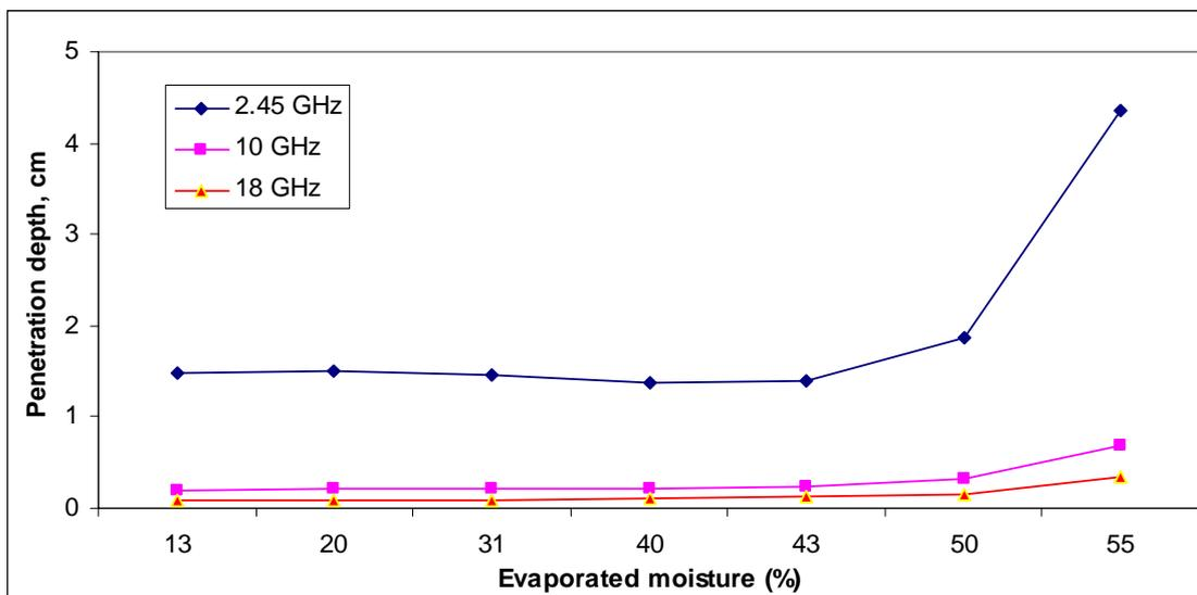
Figure 5: Penetration depth of turmeric as a function of evaporated moisture at 2.45, 10 and 18 GHz
