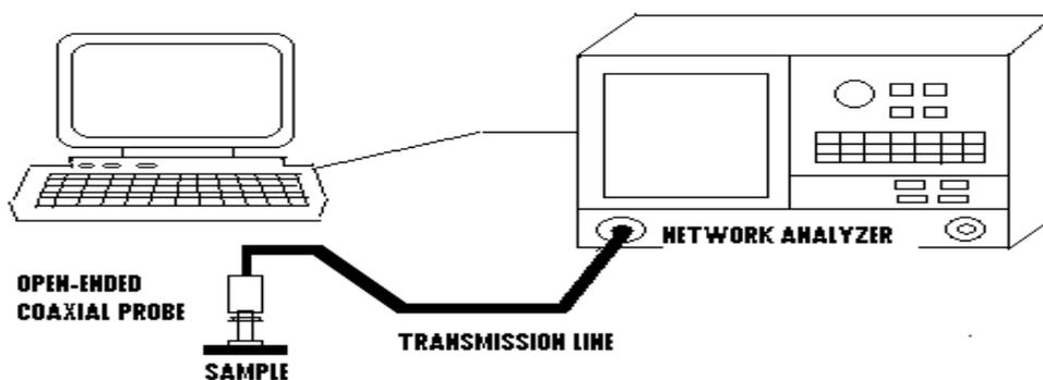
Figure 1: Schematic diagram of the dielectric measuring equipment
