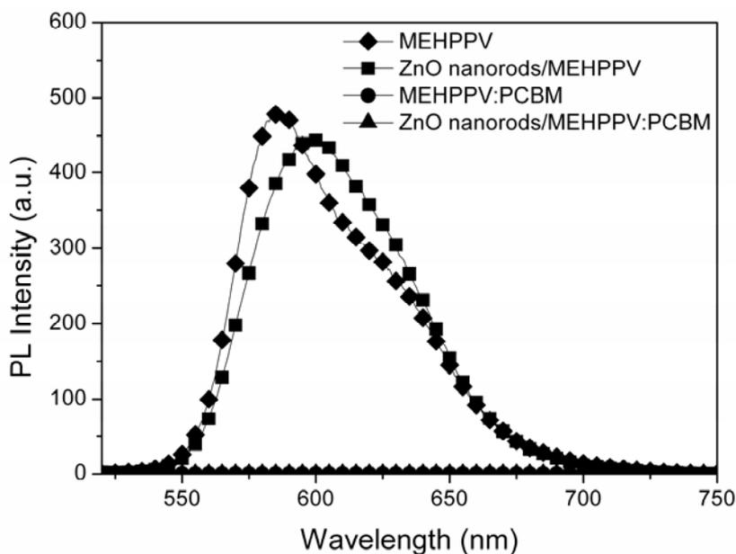
Figure 3: Photoluminescence spectra of MEHPPV, ZnO nanorods/MEHPPV hybrid film, MEHPPV:PCBM blend film and ZnO nanorods/ MEHPPV:PCBM hybrid film
