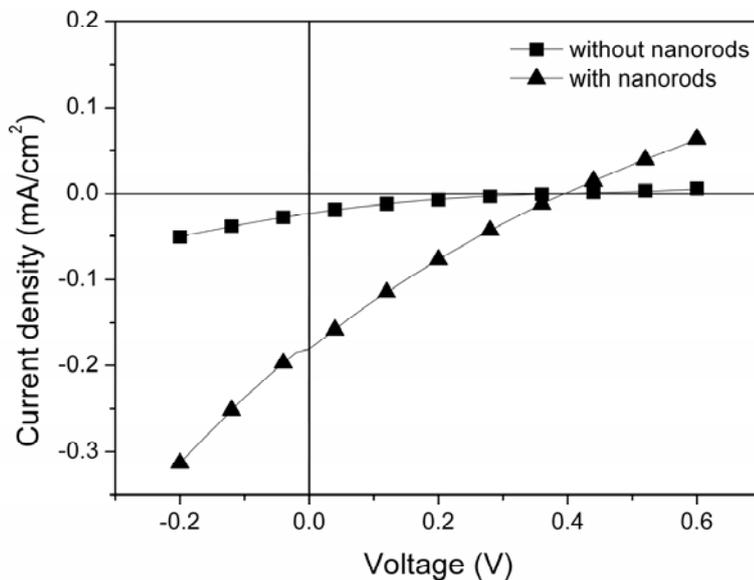
Figure 4: Current density-voltage (J-V) characteristics of solar cell without ZnO nanorods array and solar cell with ZnO nanorods array under illumination of simulated AM 1.5 G sunlight at  $100 \text{ mW/cm}^2$
