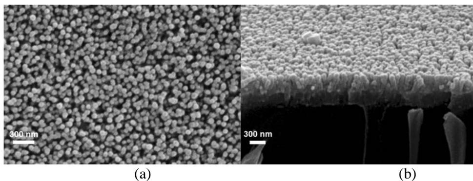
Figure 1: a) Top-view and b) cross-sectional SEM images of ZnO nanorod arrays grown on seeded-FTO substrate
