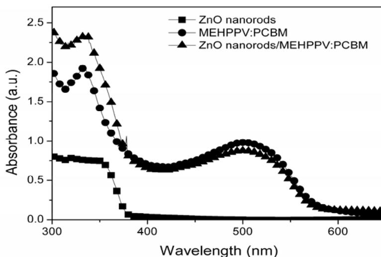
Figure 2: Absorption spectra of ZnO nanorods, MEHPPV:PCBM blend film and ZnO nanorods/MEHPPV:PCBM hybrid film
