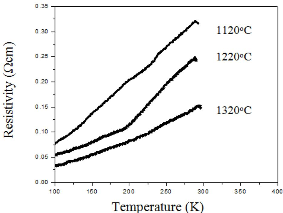
Figure 2: Resistivity versus temperature curves of  $\text{La}_{0.8}\text{Sr}_{0.2}\text{MnO}_3$
