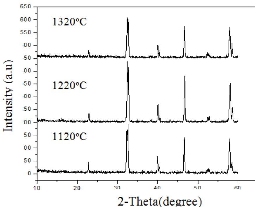
Figure 1: X-ray diffraction patterns of  $\text{La}_{0.8}\text{Sr}_{0.2}\text{MnO}_3$
