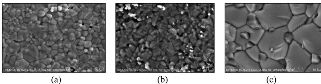
Figure 3: Scanning electron micrographs of  $\text{La}_{0.8}\text{Sr}_{0.2}\text{MnO}_3$  sintered at (a)  $1120^\circ\text{C}$ , (b)  $1220^\circ\text{C}$ , and (c)  $1320^\circ\text{C}$
