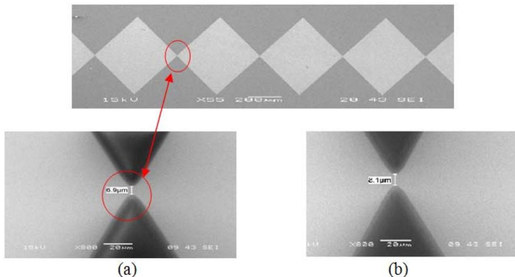
Figure 8: SEM photo show the image gap as 15 kV for sample 1:
