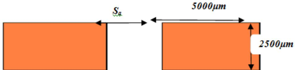
Figure 4: Design Specification for Mask 2
