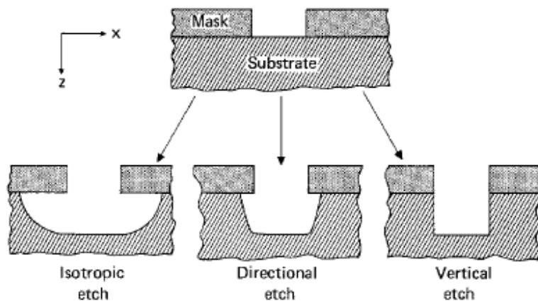
Figure1: Directionality of etching processes
