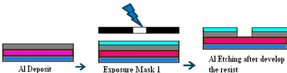
Figure 7: The first steps for nano electronic device fabrication
