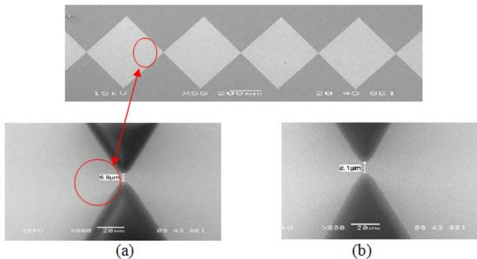
Figure 9: SEM photo show the image gap as 15 kv for sample2:
