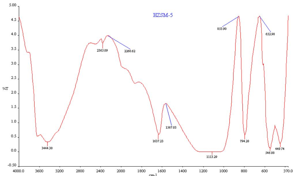
Figure 2: FTIR spectra of HZSM-5 zeolite
