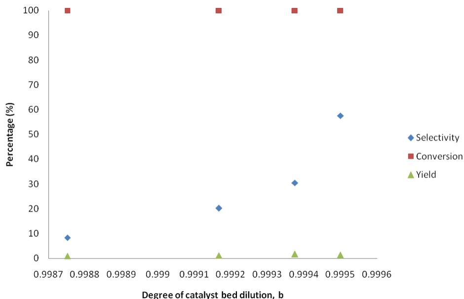
Figure 4: Conversion of glycerol, olefin selectivity and olefin yield versus degree of catalyst bed dilution
