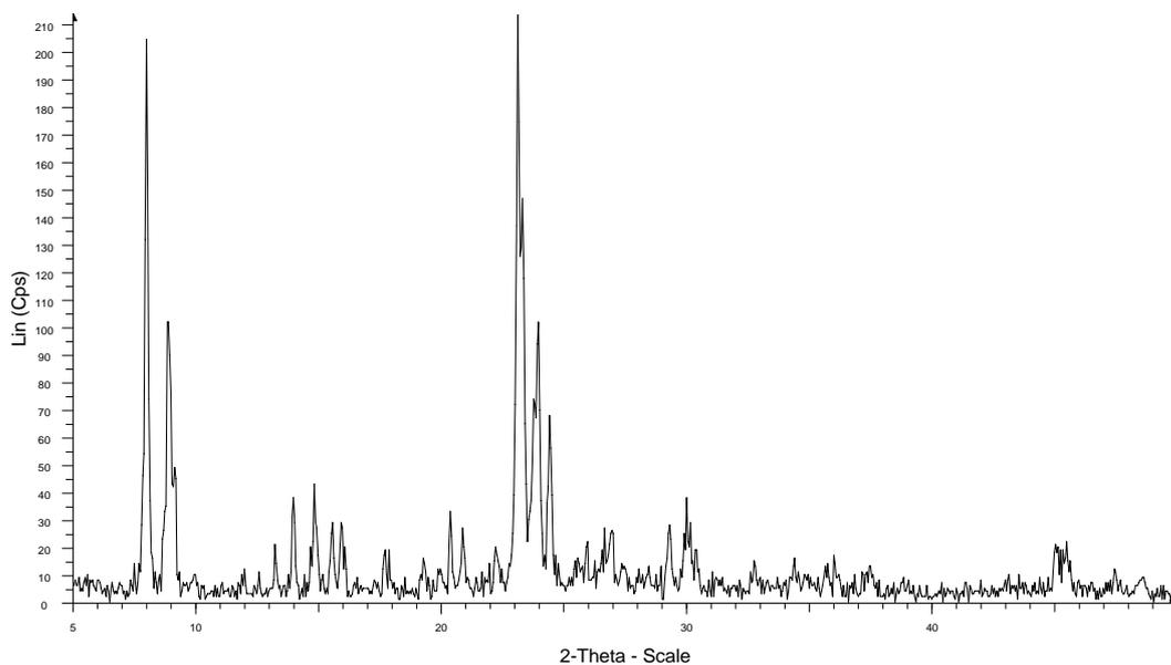
Figure 1: XRD pattern of HZSM-5 zeolite sample
