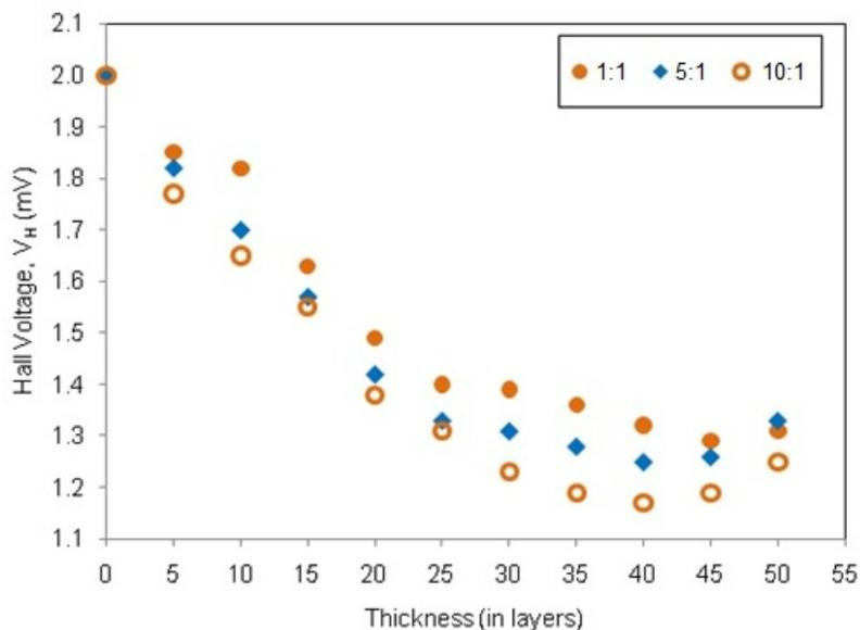
Figure 4: Hall voltage of varies PPy samples as a function of thickness
