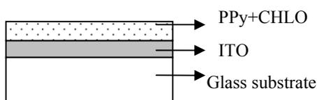
Figure 1: The structure of thin film
