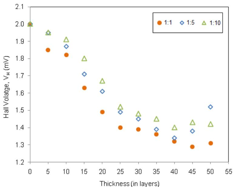
Figure 5: Hall voltage of varies CHLO with respect to the thickness
