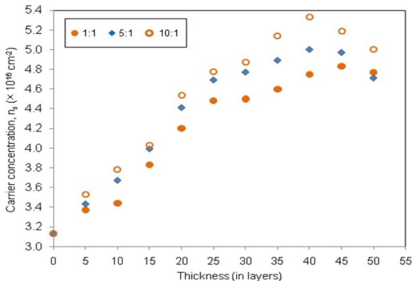
Figure 8: Carrier concentration of PPy samples film with respect to the thickness
