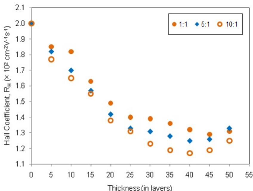
Figure 6: Hall coefficient against film thickness for varies PPy samples
