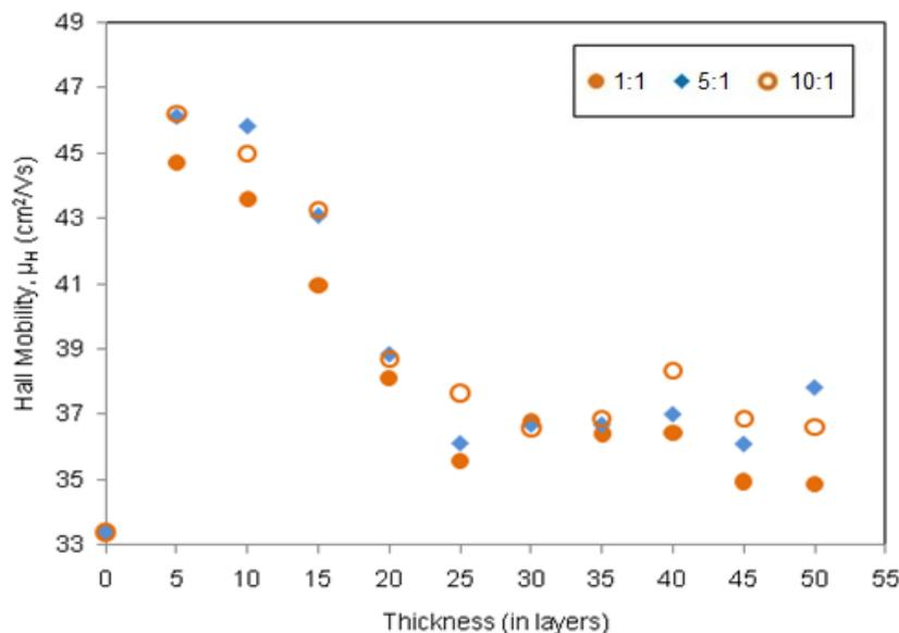
Figure 10: Hall mobility of PPy samples with respect to the thickness
