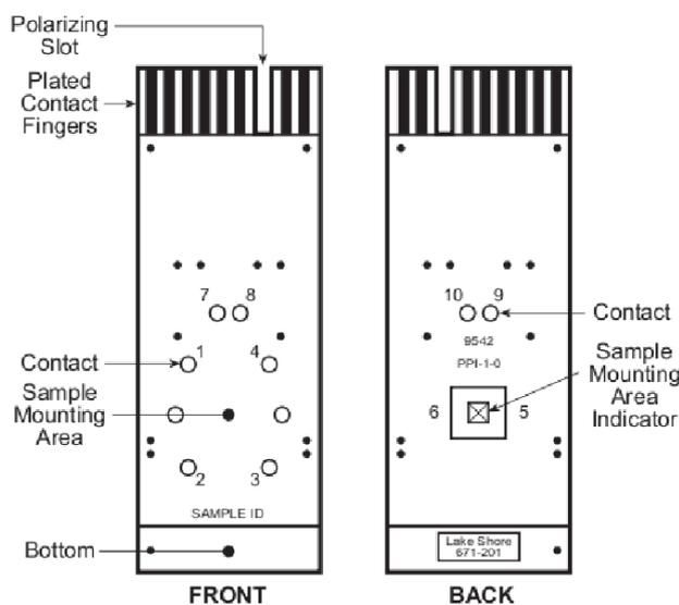
Figure 2: The geometry of sample holder [4]
