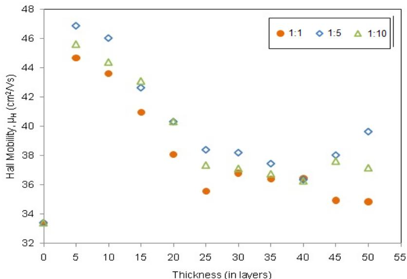
Figure 11: Hall mobility of CHLO samples with respect to the thickness
