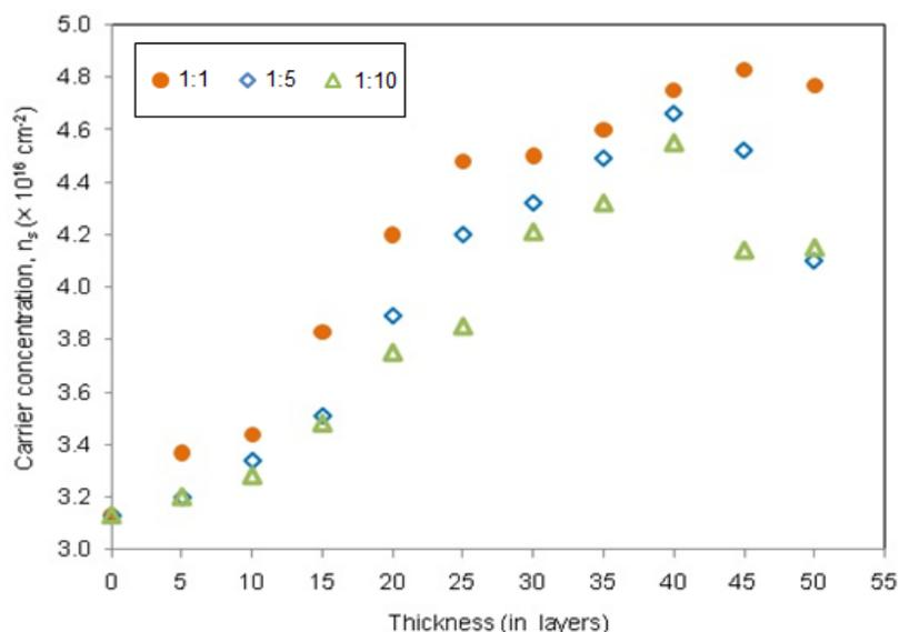
Figure 9: Carrier concentration of CHLO film with respect to the thickness
