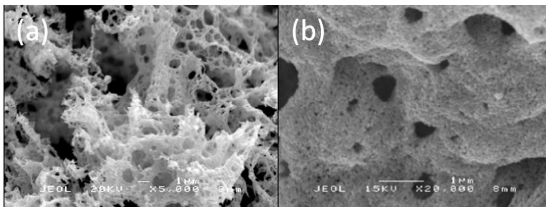
Figure 3: SEM images of the sample ID with G08400 in (a) 5000 magnification and (b) 20000 magnification
