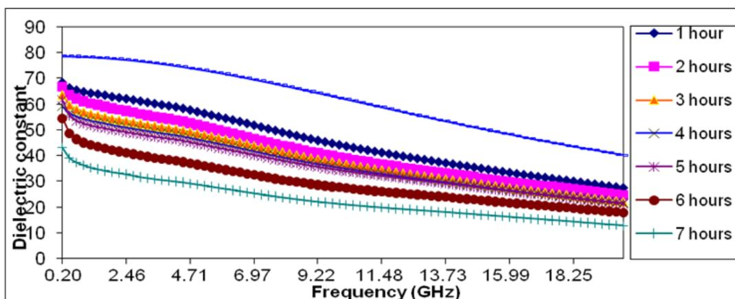
Figure 3: Dielectric constant of ginger as a function of frequency with respect to the drying times
