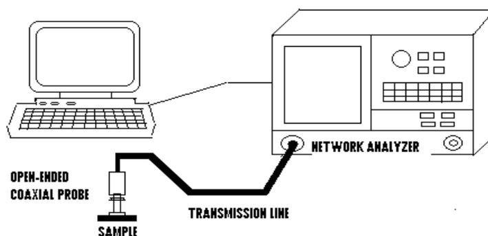
Figure 1: Schematic diagram of the dielectric measurement equipment
