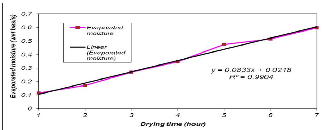
Figure 2: Evaporated moisture of ginger at various drying times
