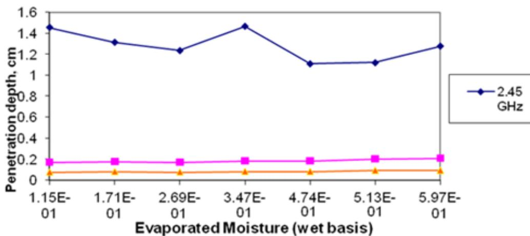
Figure 6: Power penetration depth for ginger as a function of evaporated moisture at 2.45, 10 and 18 GHz
