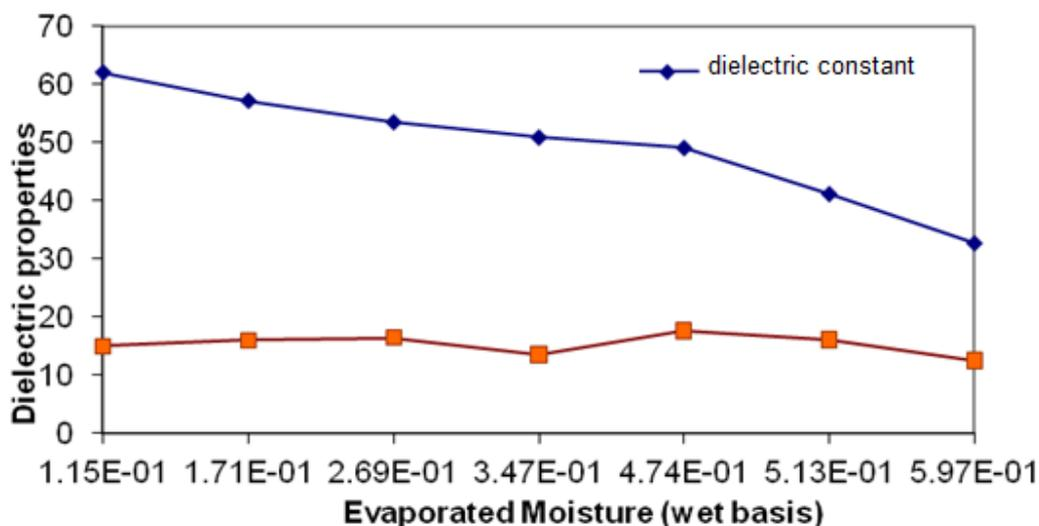
Figure 5: Dielectric properties of ginger as a function of evaporated moisture at 2.45 GHz
