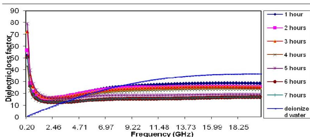
Figure 4: Dielectric loss factor of ginger as a function of frequency with respect to the drying times
