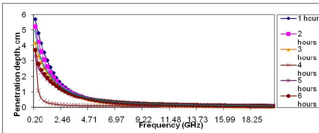
Figure 7: Power penetration depth for ginger as a function of frequency with respect to the drying times
