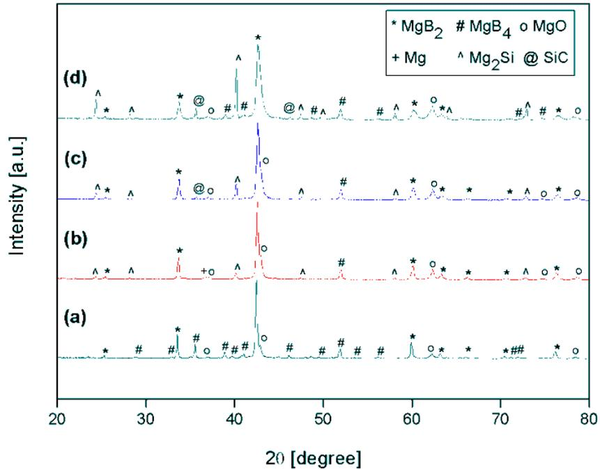
Figure 2: The XRD patterns of pure and SiC added  $Mg_{1.5}B_2$  samples sintered at  $750^\circ C$  for 4 hours
