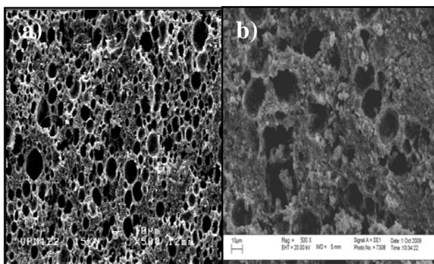
Figure 3: Microstructures of (a)  $(\text{Mg} + \text{B})$  sample and (b)  $(\text{MgB}_4 + \text{Mg})$  sample sintered at  $750\text{ }^\circ\text{C}$ . The appearance of porosity is caused by the evaporation of Mg powders
