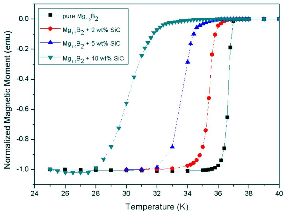
Figure 5: Normalized magnetic moment as a function of temperature for all the samples
