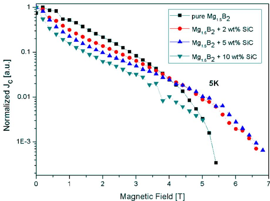
Figure 6: Normalized critical current density versus applied magnetic field,  $J_c(H)$  for all the samples at 5K
