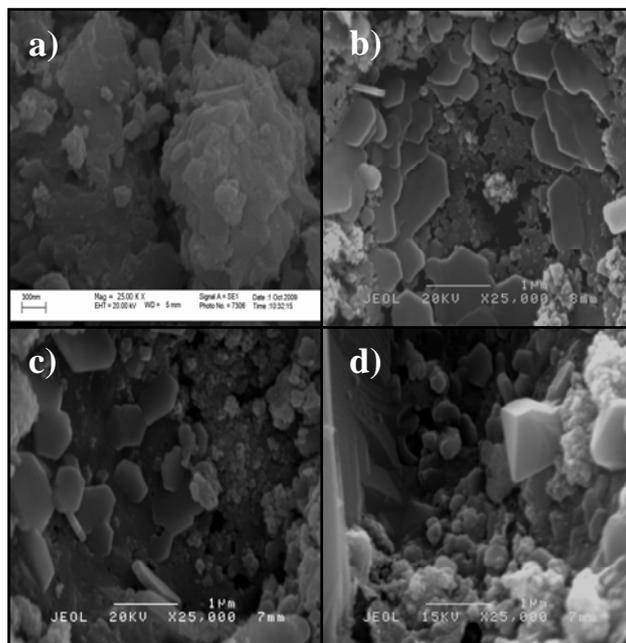
Figure 4: Scanning electron micrographs of (a) pure  $Mg_{1.5}B_2$ , (b)  $Mg_{1.5}B_2 + 2 \text{ wt\% SiC}$ , (c)  $Mg_{1.5}B_2 + 5 \text{ wt\% SiC}$  and (d)  $Mg_{1.5}B_2 + 10 \text{ wt\% SiC}$
