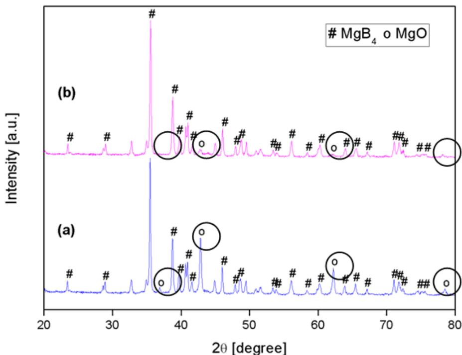
Figure 1: X-ray diffraction of MgB<sub>4</sub> powders (a) before and (b) after acid-washed
