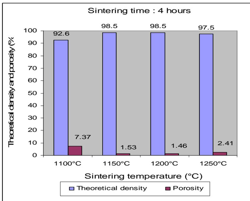
Figure 2: Effect of sintering temperature on theoretical density and porosity of Ti-6Al-4V
