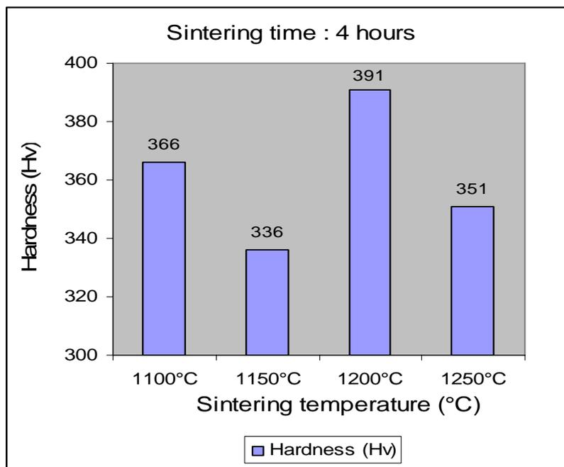
Figure 7: Effect of sintering temperatures on hardness of Ti-6Al-4V sample sintered at 1100 °C, 1150 °C, 1200 °C and 1250 °C
