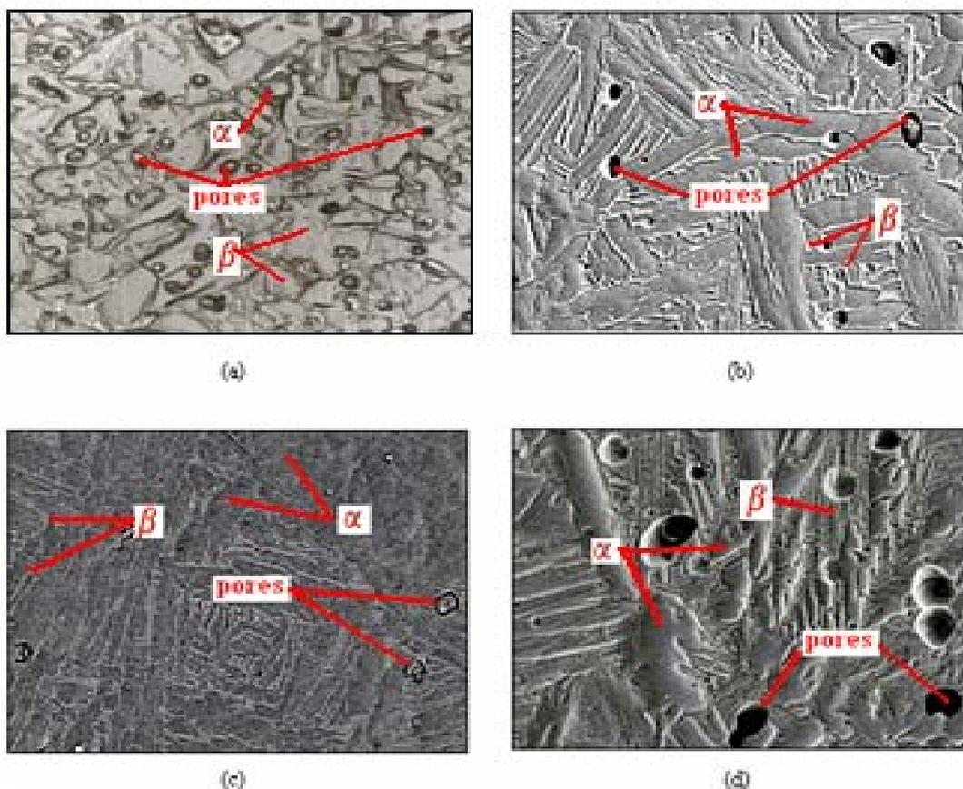
Figure 4: Microstructures of injection molded Ti-6Al-4V parts sintered at different temperatures: (a) at 1100 °C (b) at 1150 °C (c) at 1200 °C (d) at 1250 °C with heating rate dT sinter of 3.75 °Cmin<sup>-1</sup>. ( $\alpha$  = dark region  $\beta$  = white region)
