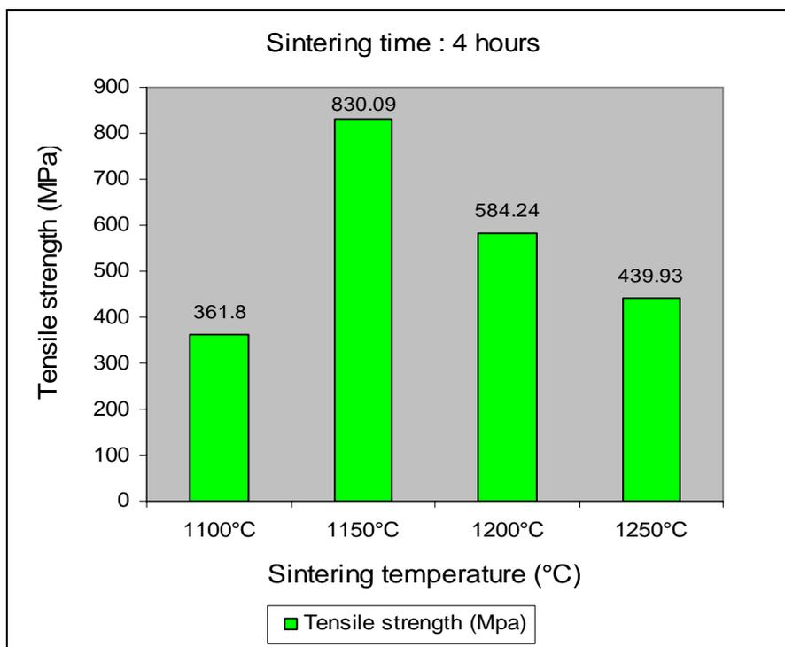
Figure 5: Effect of sintering temperature on ultimate tensile strength of Ti-6Al-4V samples sintered at 1100 °C, 1150 °C, 1200 °C and 1250 °C
