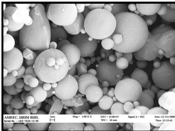
Figure 1: The morphology of Ti-6Al-4V powder
