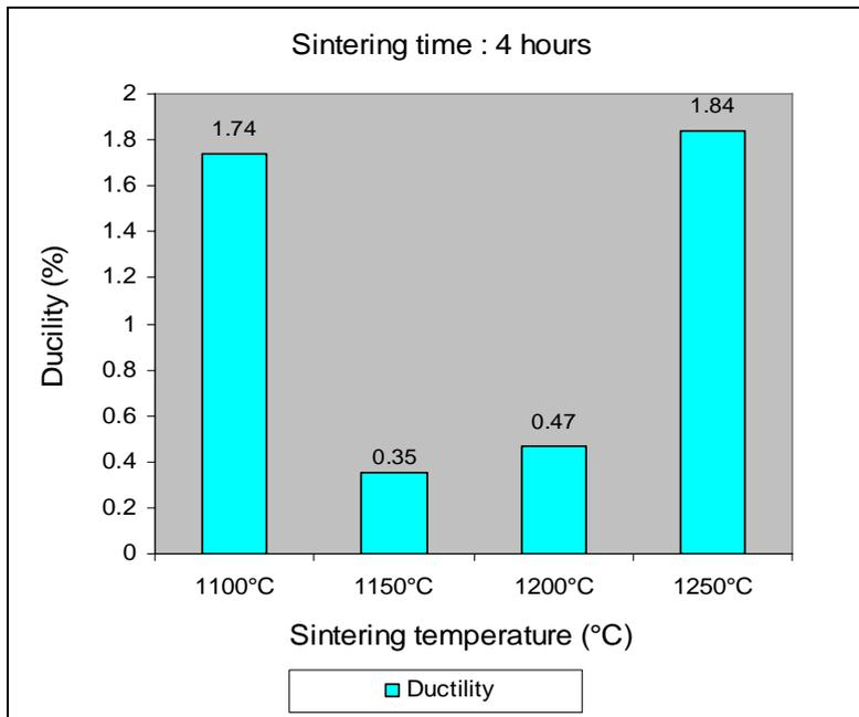
Figure 6: Effect of sintering temperatures on ductility of Ti-6Al-4V samples sintered at 1100 °C, 1150 °C, 1200 °C and 1250 °C
