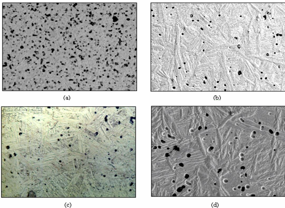
Figure 3: SEM in SE mode optical micrograph of porosity injection molded Ti-6Al-4V sintered (a) at 1100 °C (b) at 1150 °C (c) at 1200 °C (d) at 1250 °C with heating rate  $dT$  sinter of  $3.75\text{ }^{\circ}\text{Cmin}^{-1}$
