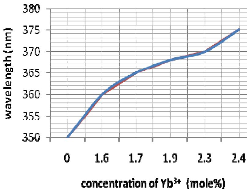
Figure 3: Cut-off wavelength (nm) against  $\text{Yb}^{3+}$
