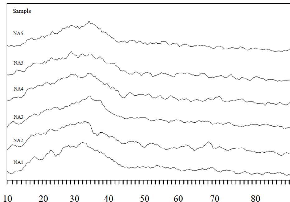
Figure 1: The X-ray diffraction (XRD) patterns of  $\text{Yb}^{3+}$  doped phosphate glass samples
