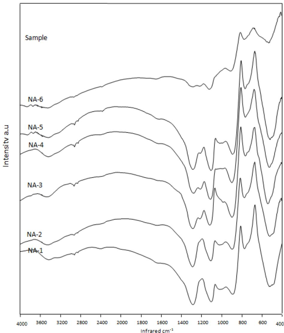
Figure 4: The Infrared spectra for  $\text{Yb}^{3+}$  doped phosphate glass samples
