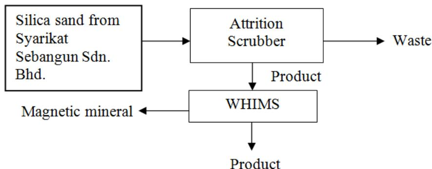
Figure 1: Flow process of upgrading silica sand
