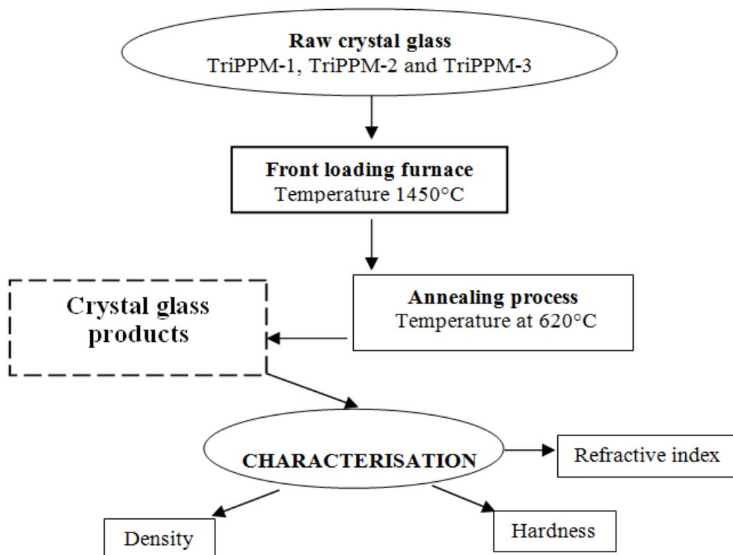
Figure 2: Flow process of melting and characterisation of crystal glass
