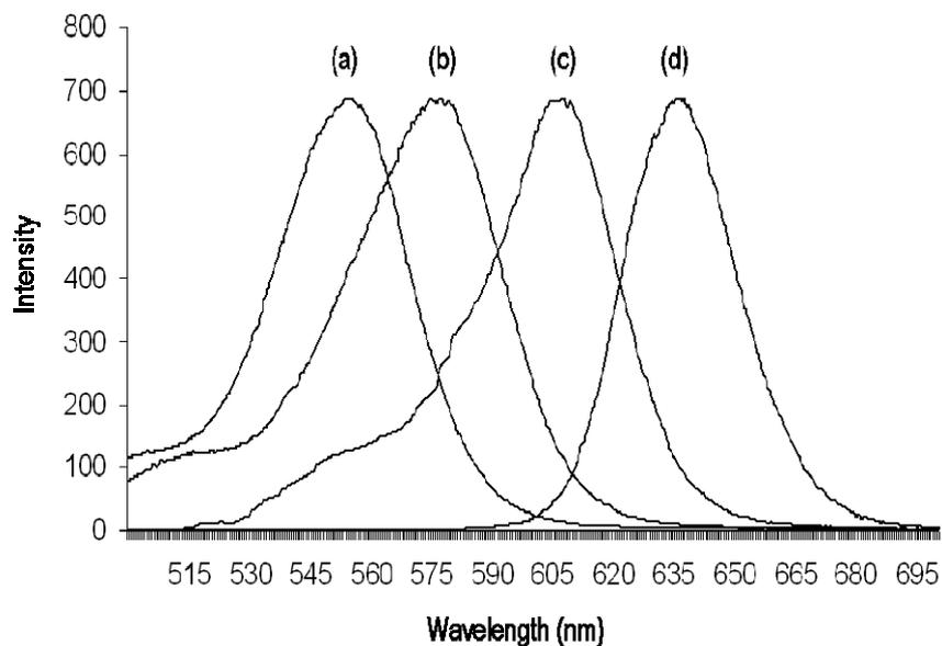
Figure 2: The photoluminescence spectra for the different temperature ranging (a) 260 °C, (b) 275 °C, (c) 290 °C and (d) 310 °C
