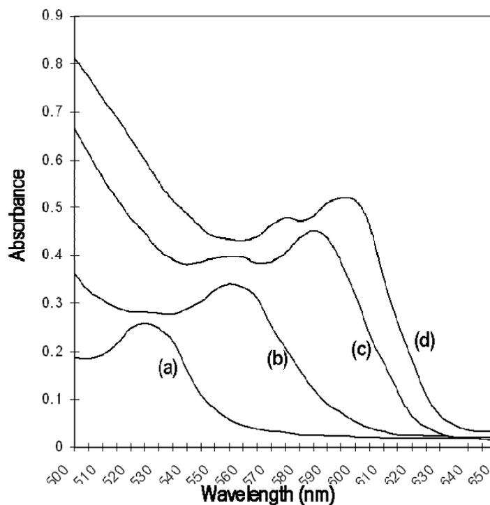
Figure 1: The UV-Vis absorption spectra for the different temperature ranging (a) 260 °C, (b) 275 °C, (c) 290 °C and (d) 310 °C
