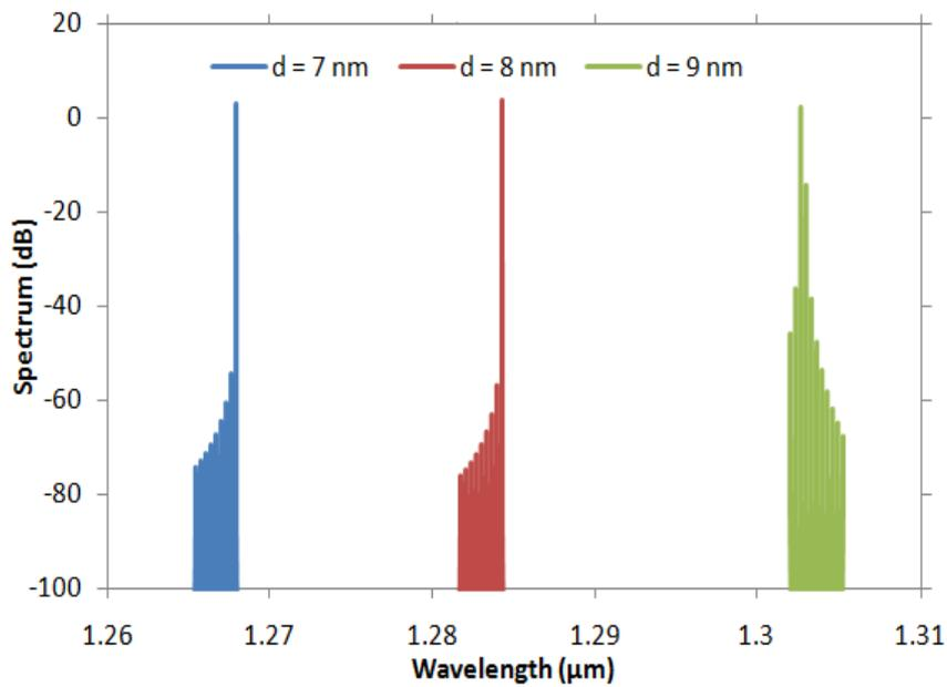
Figure 4: The mode spectrum with different quantum well thicknesses (7 nm, 8 nm and 9 nm)
