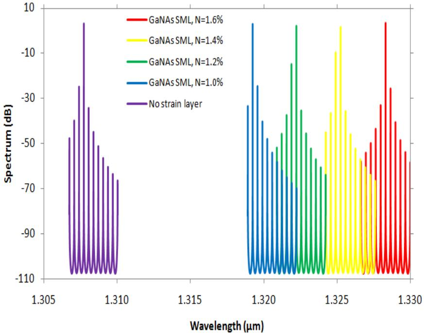
Figure 5: The mode spectrum with different nitrogen percentage in the quantum well layer (1.6%, 1.4%, 1.2% and 1.0%)
