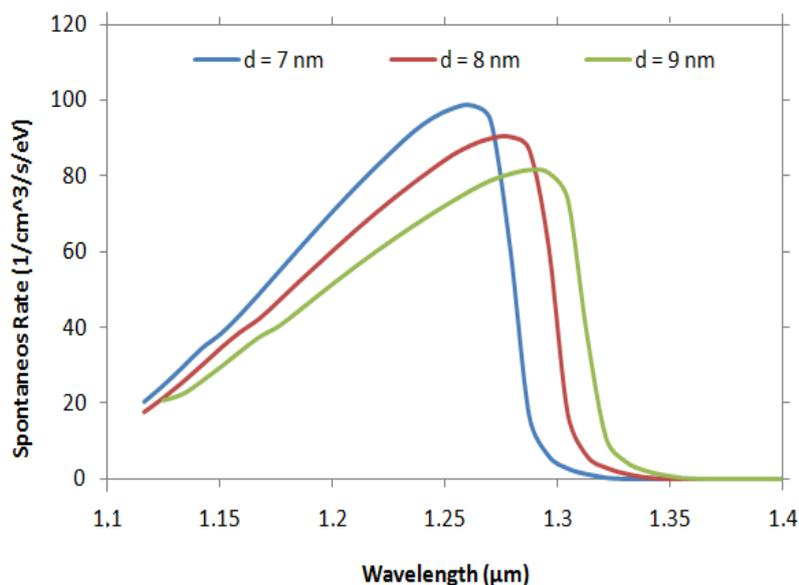
Figure 3: Photoluminescence spectrum with different quantum well thicknesses (7 nm, 8 nm and 9 nm)
