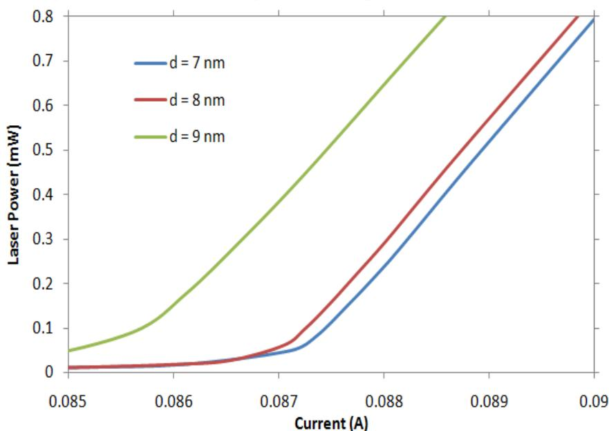
Figure 6: Threshold current ( $I_{th}$ ) with different quantum well thicknesses (7 nm, 8 nm and 9 nm)
