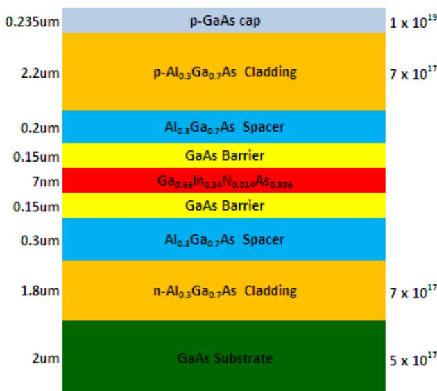
Figure 1: The schematic cross-section of the device structure
