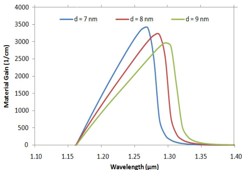
Figure 2: Gain material spectrum with different quantum well thicknesses (7 nm, 8 nm and 9 nm)
