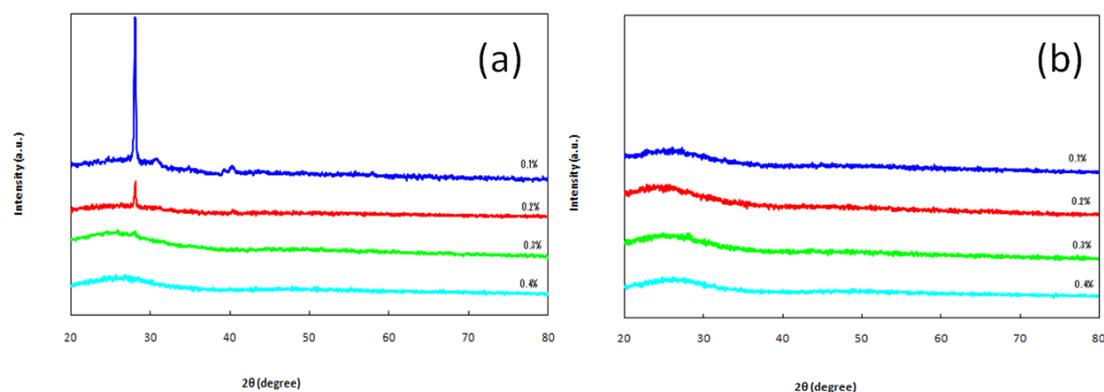
Figure 1. The XRD patterns for MnO–B<sub>2</sub>O<sub>3</sub>–TeO<sub>2</sub> glasses (a) original sample, and (b) remelted sample
