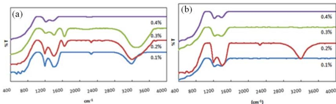
Figure 4: FT-IR spectra of (a) original sample (b) remelted sample
