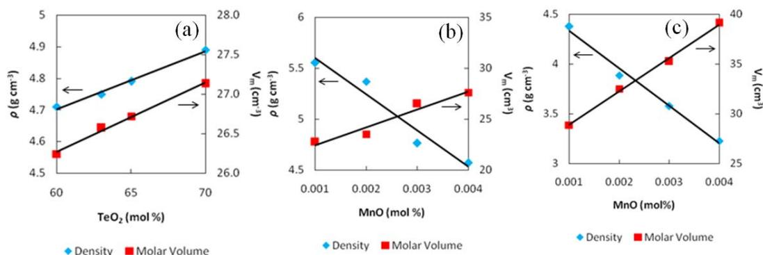
Figure 3: Density and molar volume comparison of (a) borotellurite glasses, (b) original sample and (c) remelted sample
