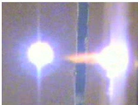
Figure 4: Pre-formed plasma, plasma jet and aluminum plasma plume during interaction with aluminum target
