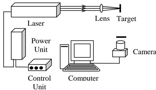
Figure 2: Experimental setup of IR laser plasma interaction with aluminum target
