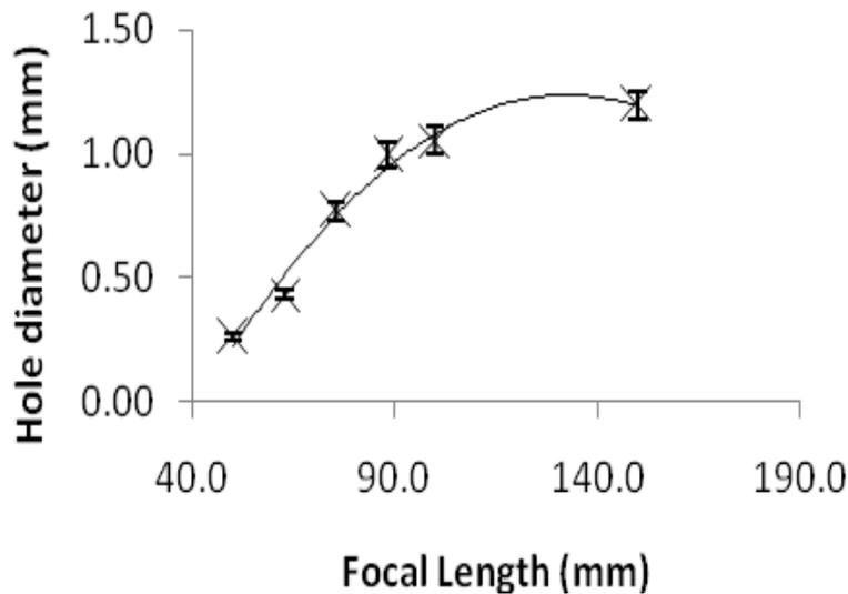
Figure 5: Hole size on aluminum target as a function of lens focal length
