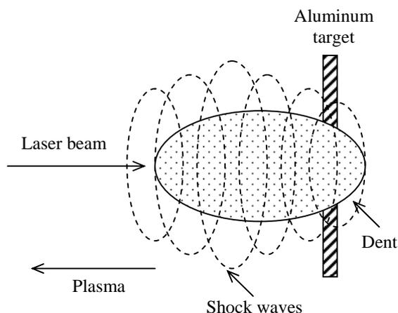
Figure 7: Plasma generation associated with shock waves impinges on aluminum
