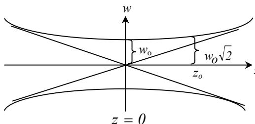
Figure 1: Laser beam in the form of Gaussian beam after been focused by lens. At a focal point,  $z = 0$ , the beam waist is  $w_o$  and at Rayleigh region  $z_o$  the beam waist is extend to  $w_o\sqrt{2}$
