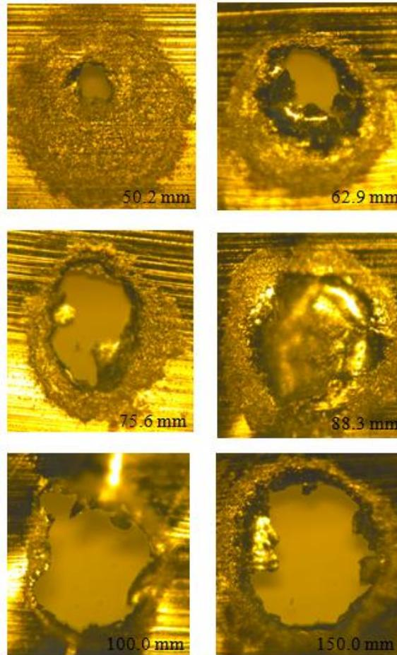
Figure 3: Images of laser plasma interaction with aluminum target
