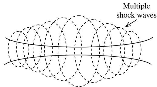
Figure 6: Multiple shock waves induced when the pulsed laser beam is brought by a lens
