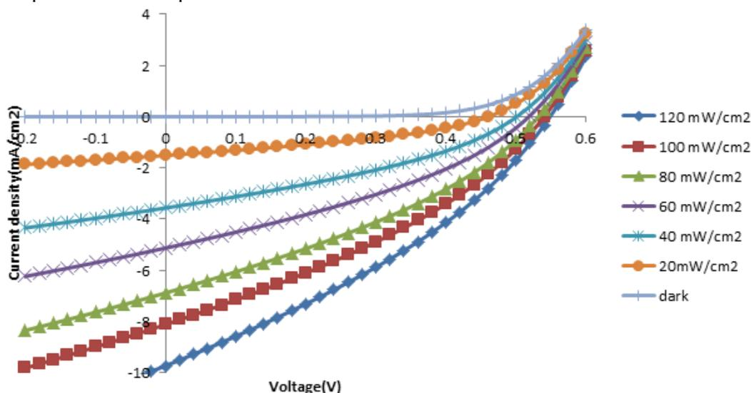
Figure 2: SCAPS simulation of the I-V curves of a Al/LiF/P3HT : PCBM /ITO/PEDOT-PSS solar cell, for varying illumination intensity
