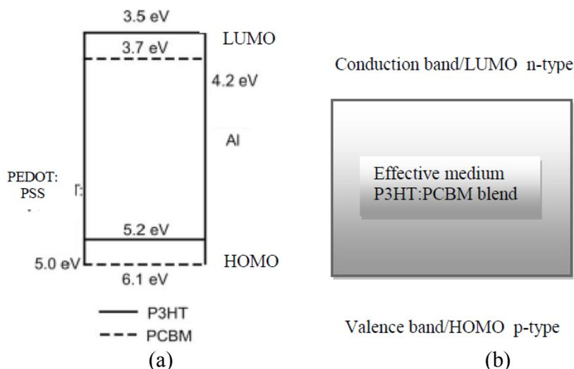
Figure 1: (a) Schematic energy level diagrams of the PEDOT:PSS/ P3HT:PCBM/Al solar cell before the materials are brought into intimate contact; (b) the effective medium model which the intimate blend of an *n*-type material and a *p*-type material is represented by one single 'effective' material with 'average' properties
