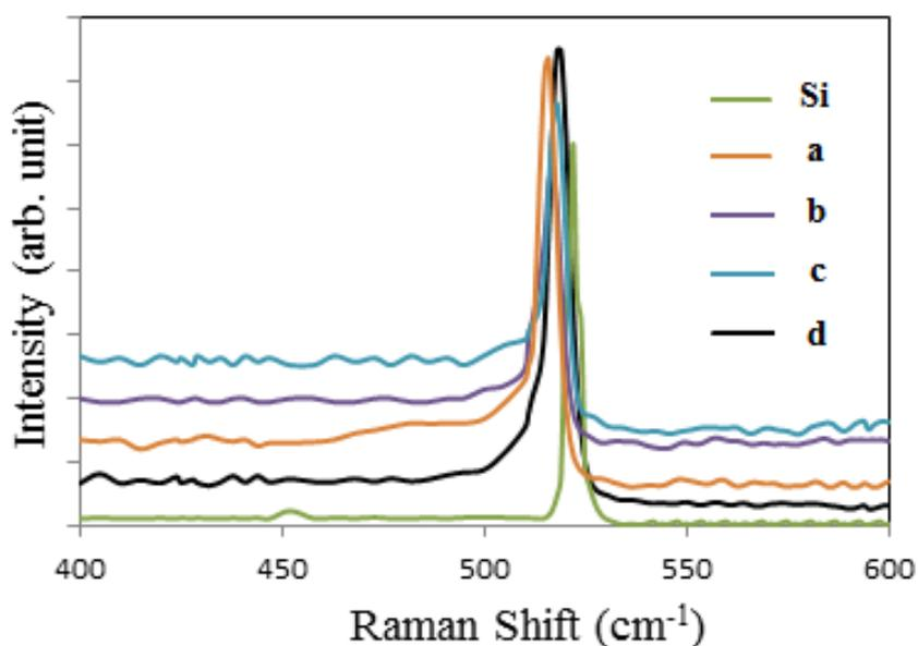
Figure 4: Raman spectra of the SiNWs fabricated using PECVD at various Silane flow rate; a) 5 sccm b) 10 sccm c) 15 sccm d) 20 sccm
