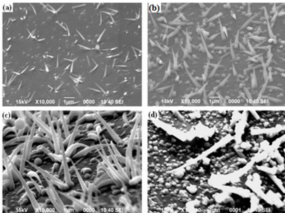
Figure 1: SEM images of silicon nanowires grown at 450 °C and various silane gas flow rate; a) 5 sccm b) 10 sccm c) 15 sccm d) 20 sccm
