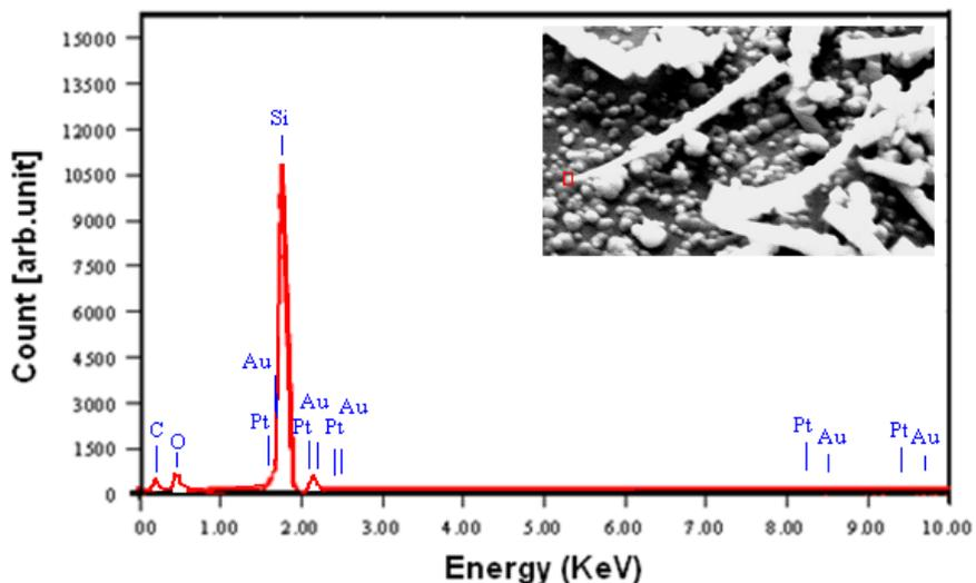
Figure 2: The EDX spectrum of a silicon nanowire grown at 450 °C and 20 sccm
