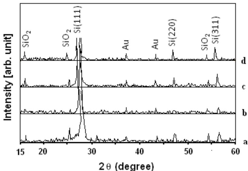
Figure 3: XRD patterns of the SiNWs on Si (111) substrate at various silane gas flow rate: (a) 5 sccm, (b) 10 sccm, (c) 15 sccm, and (d) 20 sccm
