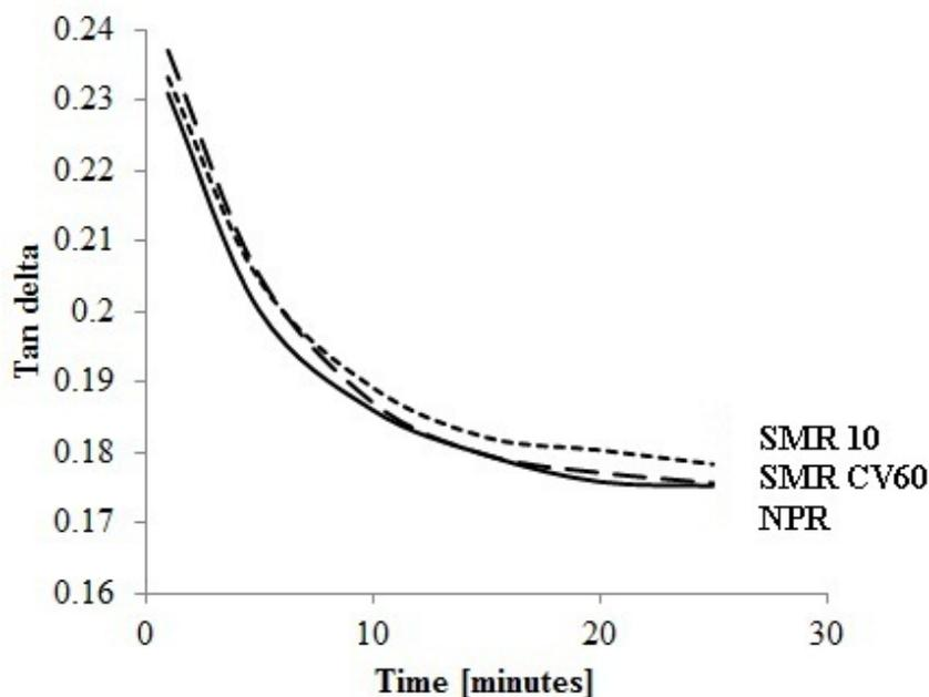
Figure 4: Effect of test duration on tan delta tested at 55°C
