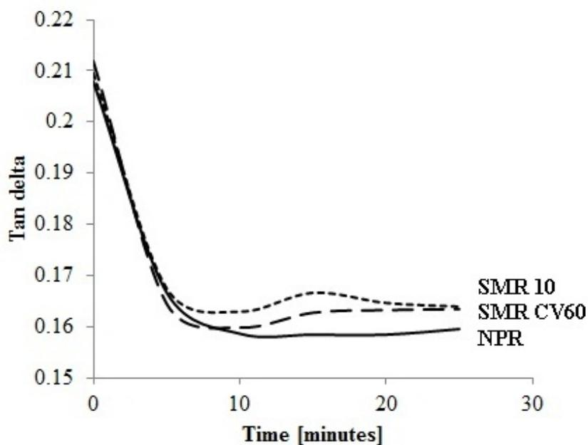
Figure 5: Effect of test duration on tan delta tested at 100°C
