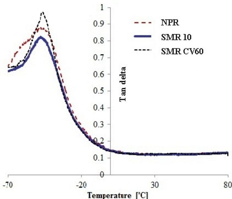
Figure 1: Dynamic properties of vulcanisates by DMTA
