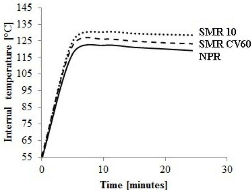
Figure 2: Effect of test duration on temperature (internal sample) tested at 55°C
